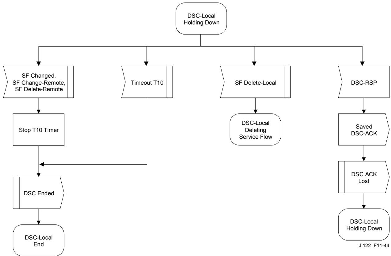
**Figure 11-44/J.122 – DSC – Locally initiated Transaction Holding Down State Flow Diagram**
