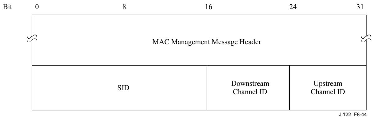
**Figure 8-44/J.122 – Packet PDU following the Timing Header**
