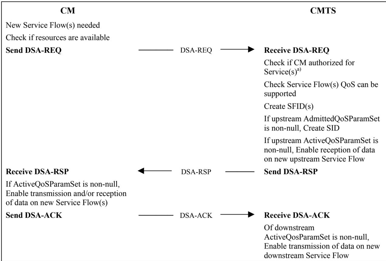
a) Authorization can happen prior to the DSA-REQ being received by the CMTS. The details of CMTS signalling to anticipate a DSA-REQ are beyond the scope of this Recommendation.
