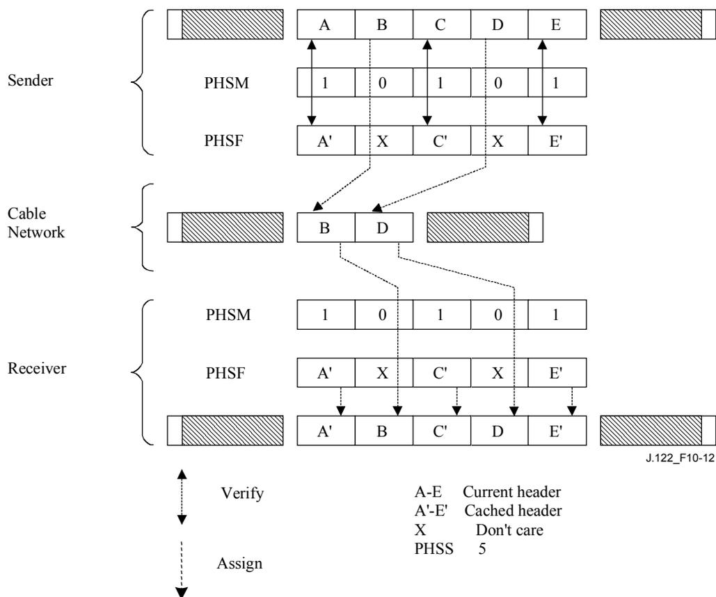
**Figure 10-12/J.122 – Payload Header Suppression with Masking**
