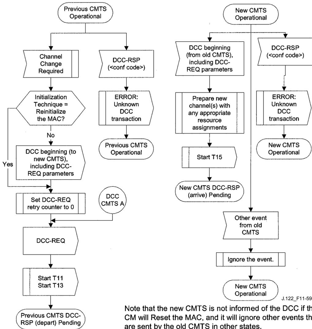
Figure 11-59/J.122 – Dynamically changing channels: CMTS view, Part 1
