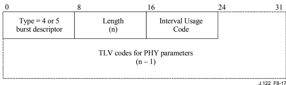
**Figure 8-17/J.122 – Top-level encoding for burst descriptors**
