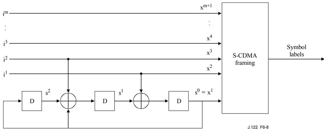
**Figure 6-8/J.122 – Convolutional encoder**
