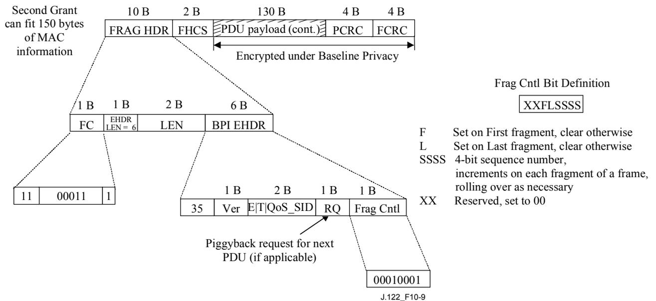
Figure 10-9/J.122 – Example of fragmenting a single packet
