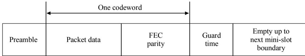
Example 2) Packet length = k + remaining information bytes in 2nd codeword = k + k' ≤ k + k'' ≤ 2k
