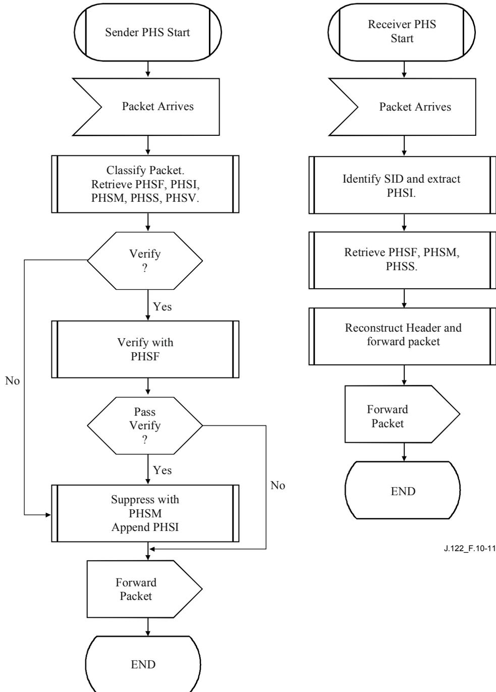
**Figure 10-11/J.122 – Payload Header Suppression operation**
