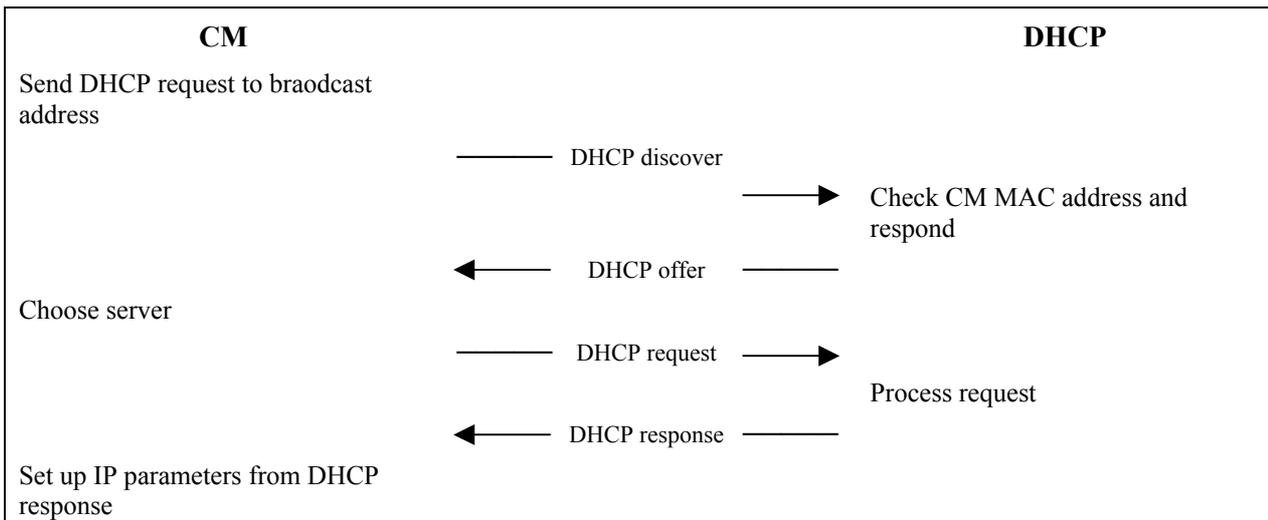
**Figure 11-10/J.122 – Establishing IP connectivity**
