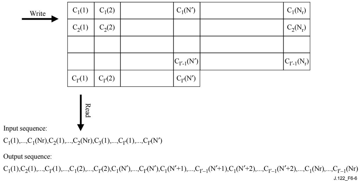
**Figure 6-6/J.122 – Interleaver operation for last Interleaver block (with shortened last codeword)**
