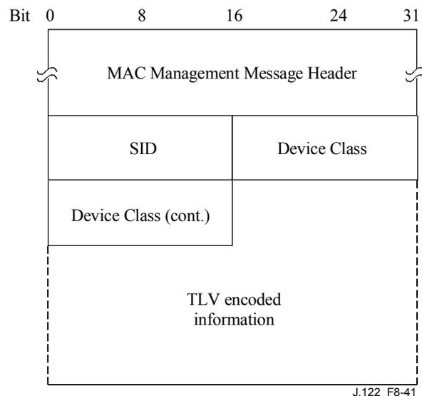
Figure 8-41/J.122 – Device Class Identification Request
