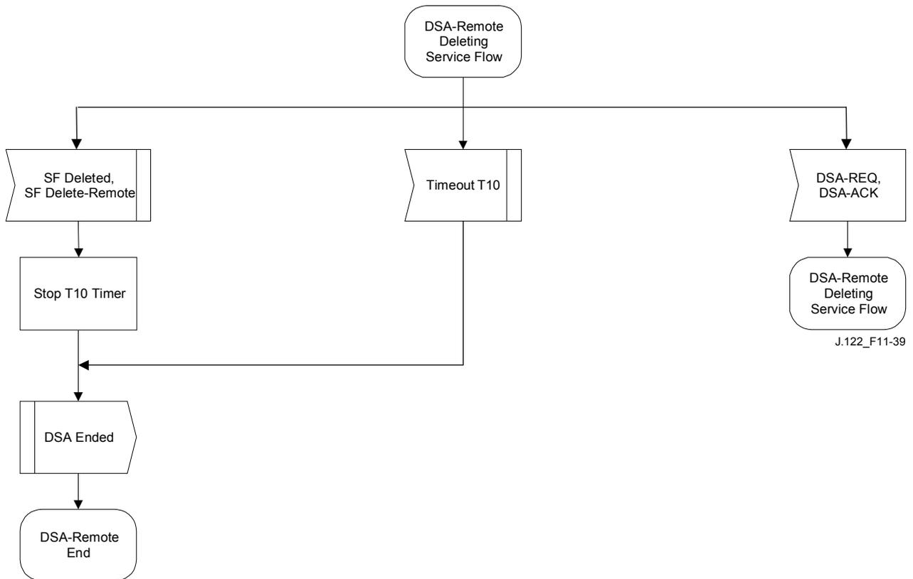
**Figure 11-39/J.122 – DSA – Remotely initiated Transaction Deleting Service State Flow Diagram**
