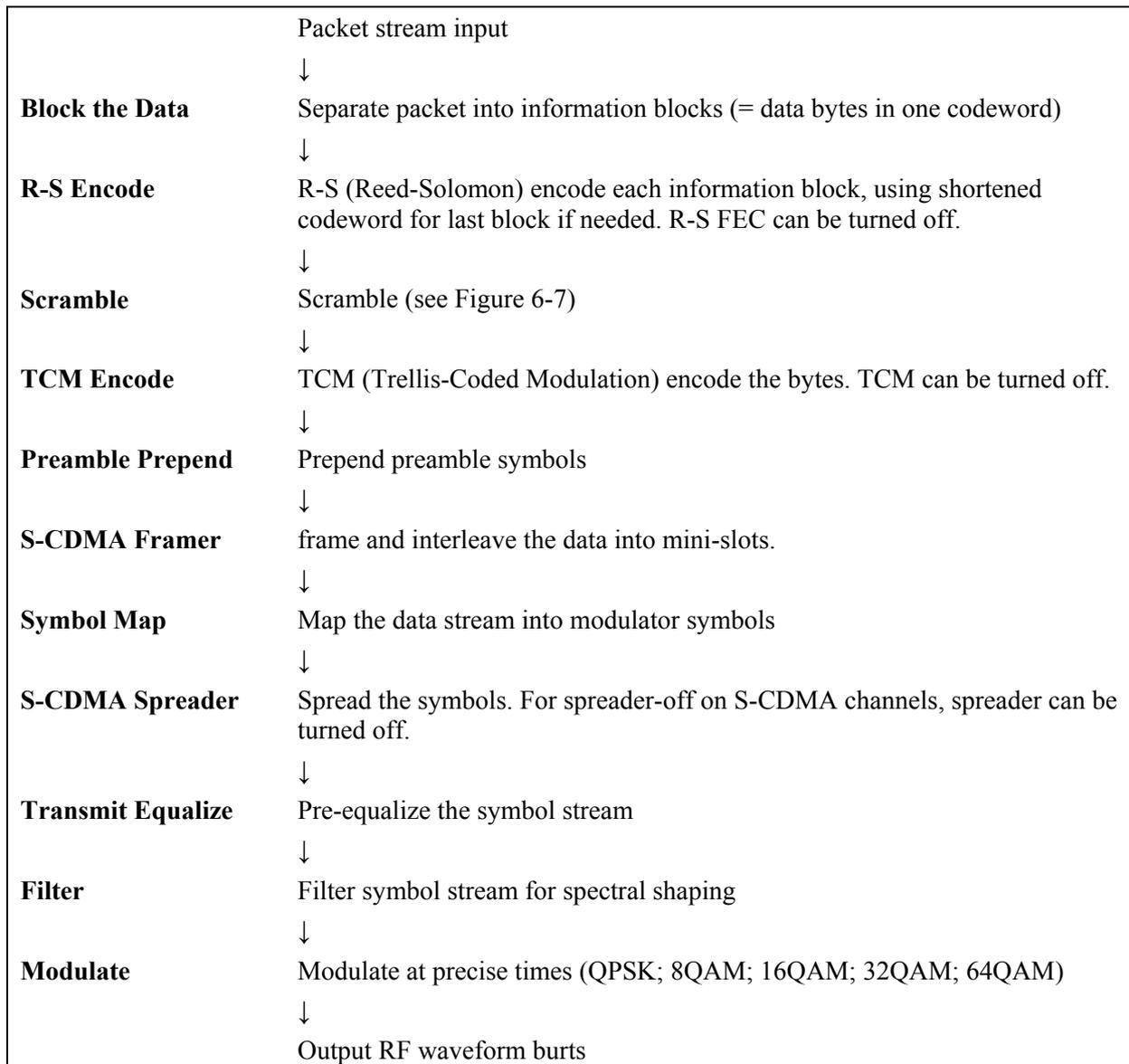
**Figure 6-3/J.122 – S-CDMA upstream transmission processing**
