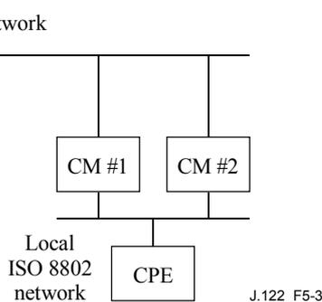
**Figure 5-3/J.122 – Example condition for network loops**
