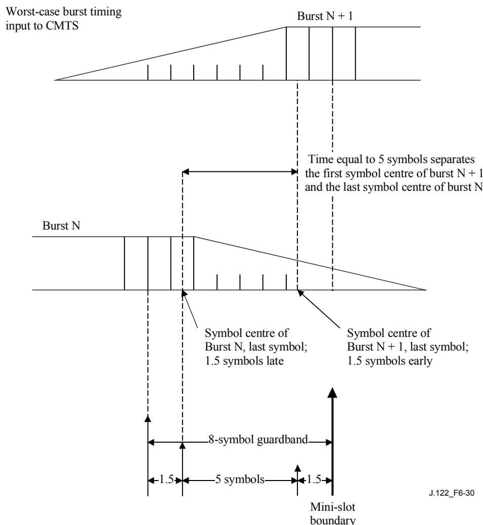
**Figure 6-30/J.122 – Worst-case TDMA burst timing**
