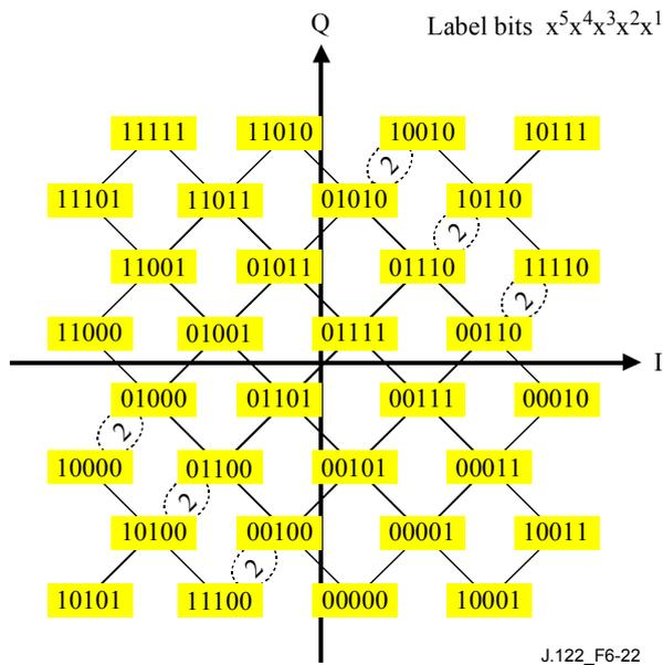
**Figure 6-22/J.122 – 32QAM symbol mapping**
