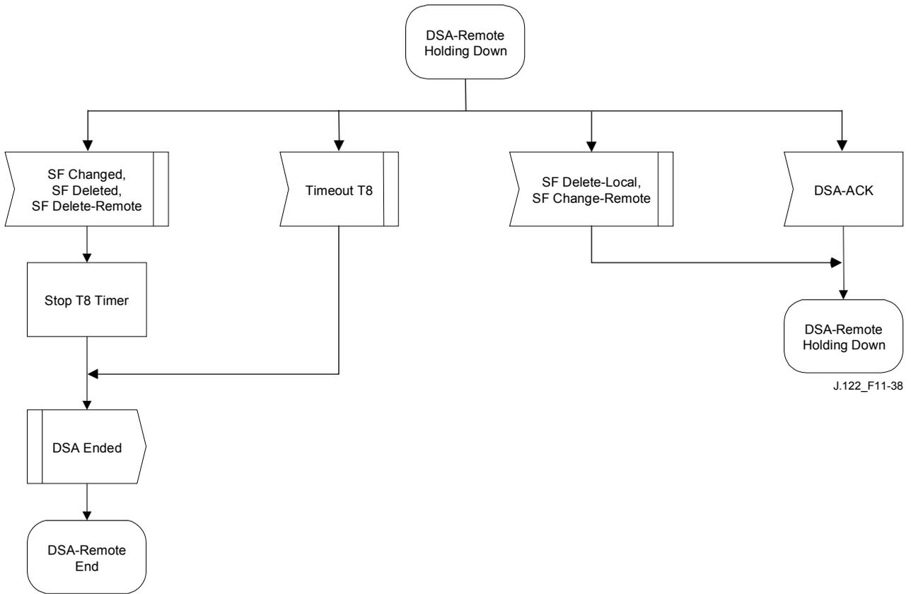
**Figure 11-38/J.122 – DSA – Remotely initiated Transaction Holding Down State Flow Diagram**
