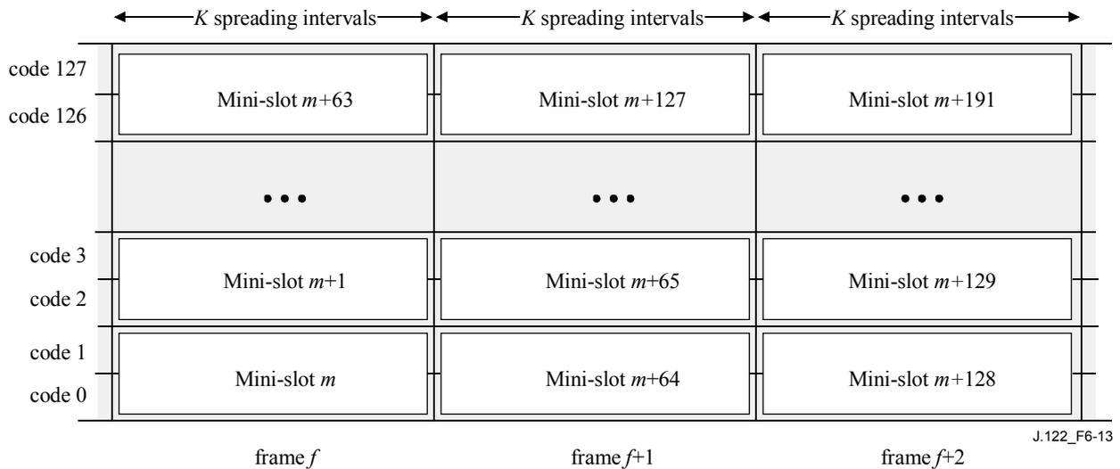
**Figure 6-13/J.122 – Mini-slot mapping with two codes per mini-slot, 128 active codes**
