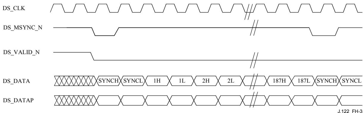
**Figure H.3/J.122 – Downstream Data Signal Protocol For J.83 Annex B Operation**
