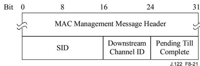
Figure 8-21/J.122 – Packet PDU following the Timing Header
