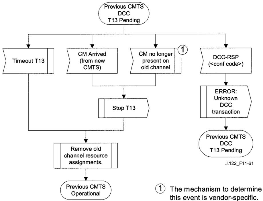
**Figure 11-61/J.122 – Dynamically changing channels: CMTS view, Part 3**
