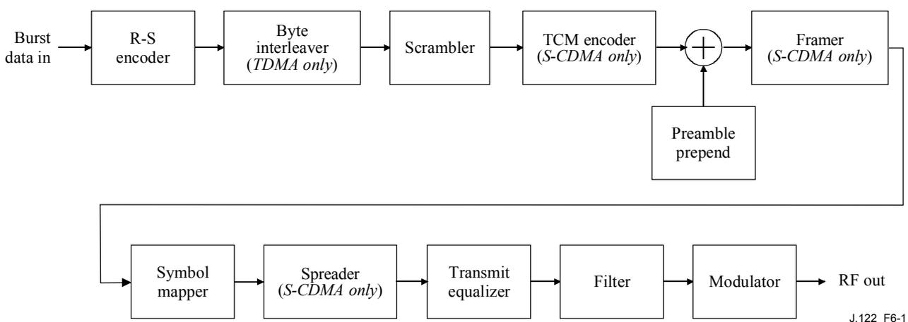
**Figure 6-1/J.122 – Upstream signal-processing sequence**
