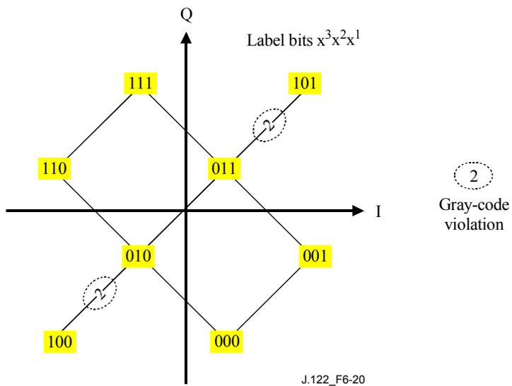
**Figure 6-20/J.122 – 8QAM symbol mapping**
