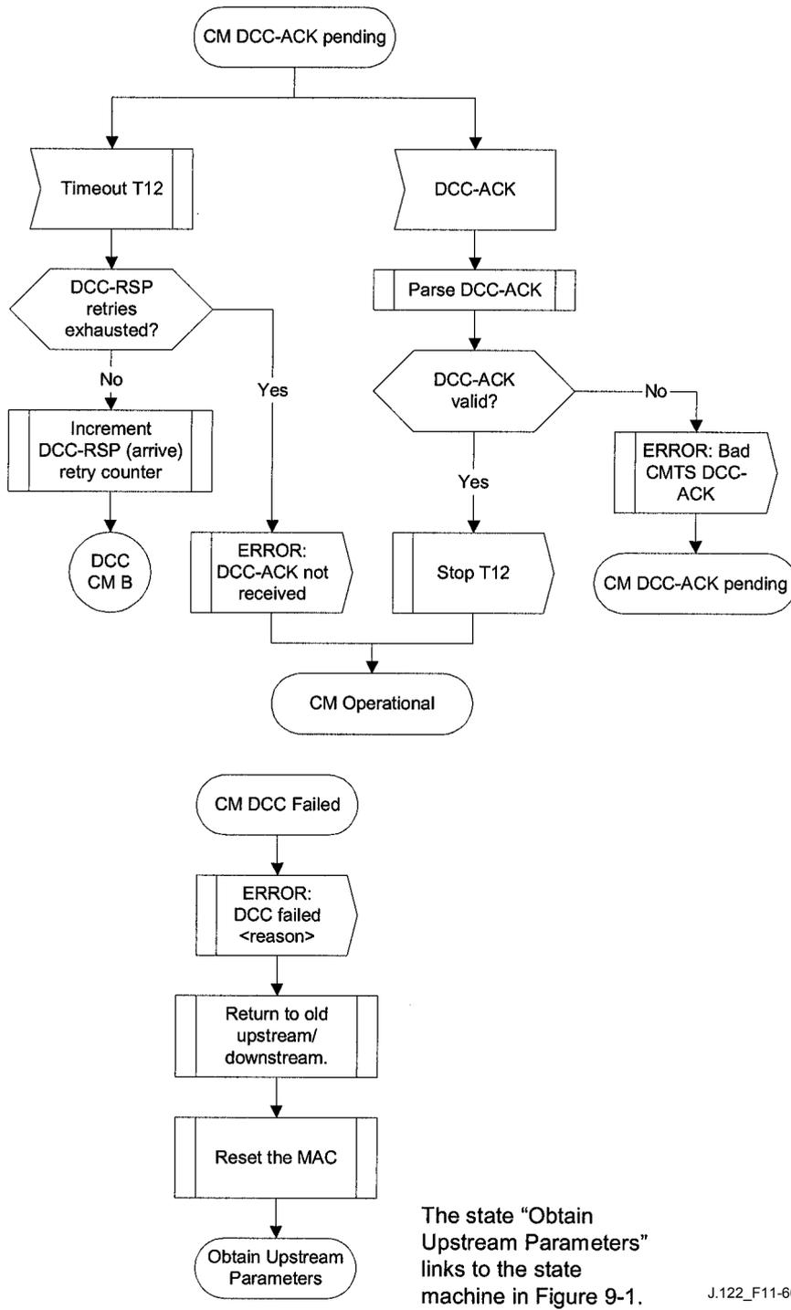
Figure 11-66/J.122 – Dynamically changing channels: CM view, Part 4
