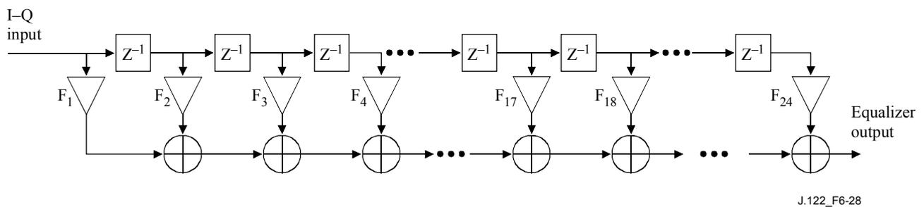
**Figure 6-28/J.122 – Transmit pre-equalizer structure**
