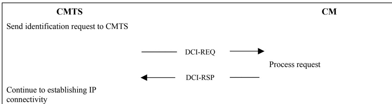
**Figure 11-9/J.122 – Device Class identification**
