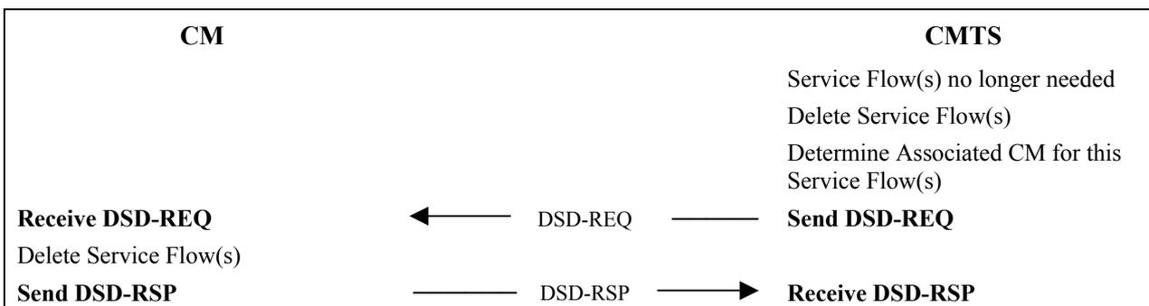
**Figure 11-52/J.122 – Dynamic Service Deletion initiated from CMTS**
