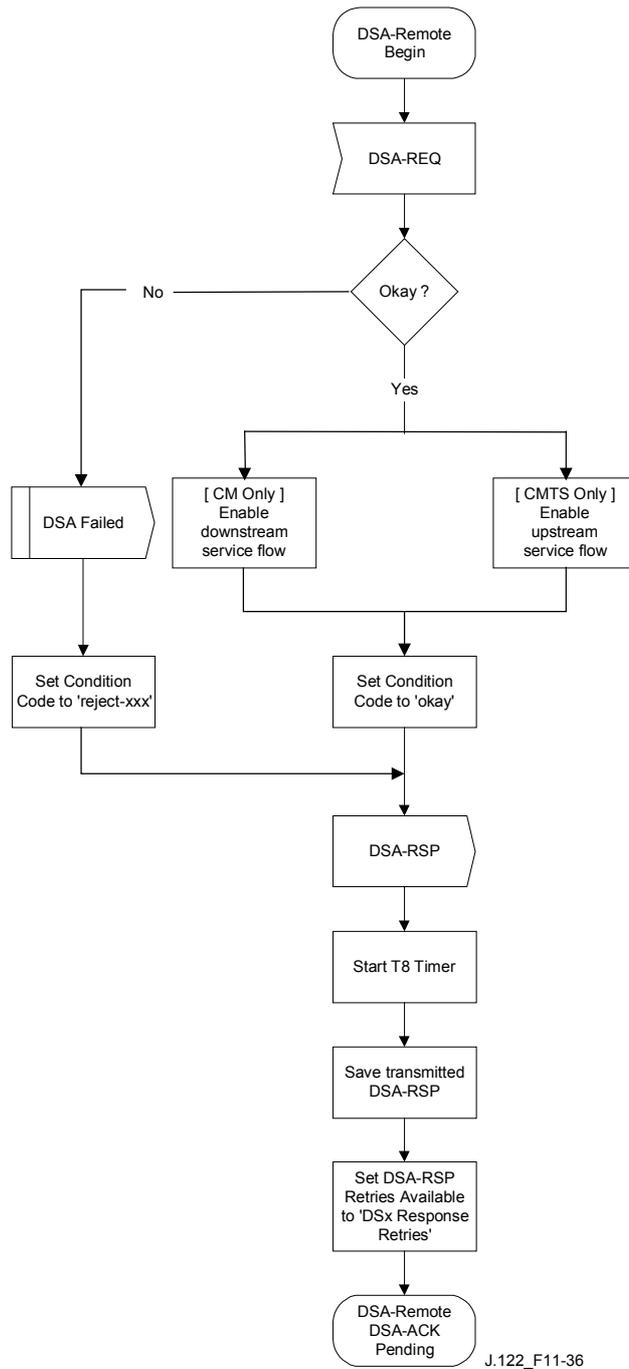
**Figure 11-36/J.122 – DSA – Remotely initiated Transaction Begin State Flow Diagram**
