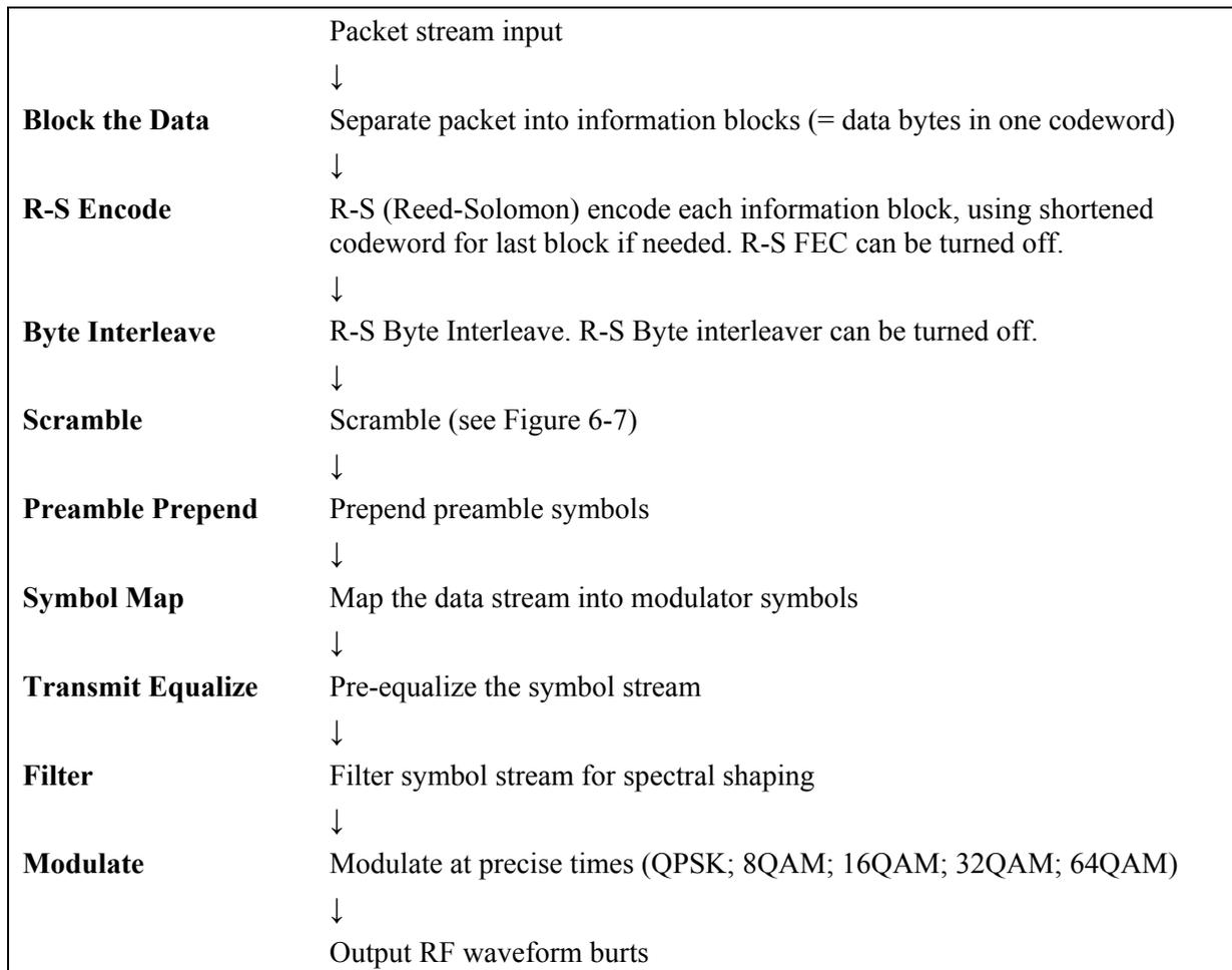
**Figure 6-2/J.122 – TDMA upstream transmission processing**
