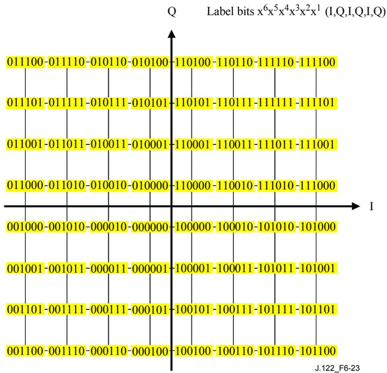
**Figure 6-23/J.122 – 64QAM symbol mapping**
