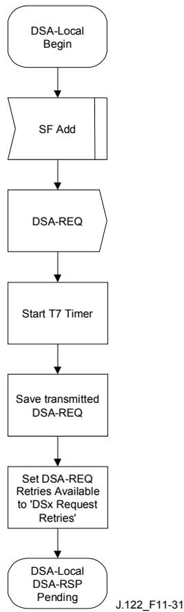
Figure 11-31/J.122 – DSA – Locally initiated Transaction Begin State Flow Diagram
