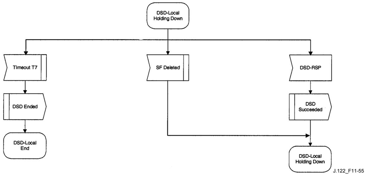
**Figure 11-55/J.122 – DSD – Locally initiated Transaction Holding Down State Flow Diagram**
