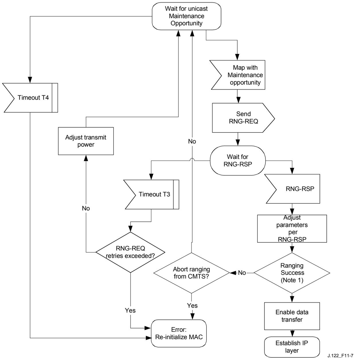
NOTE 1 – Ranging Request is within the tolerance of the CMTS.
