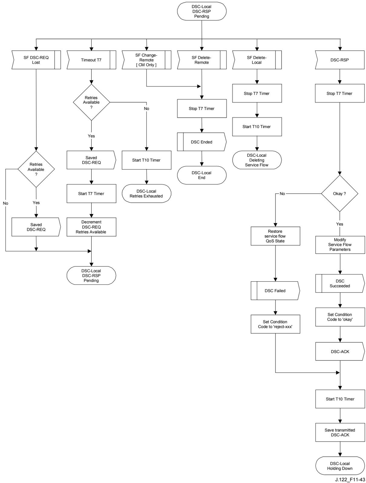
**Figure 11-43/J.122 – DSC – Locally initiated Transaction DSC-RSP Pending State Flow Diagram**
