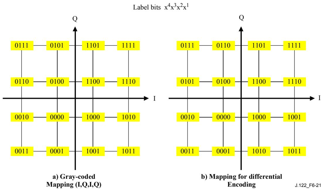
**Figure 6-21/J.122 – 16QAM symbol mapping**
