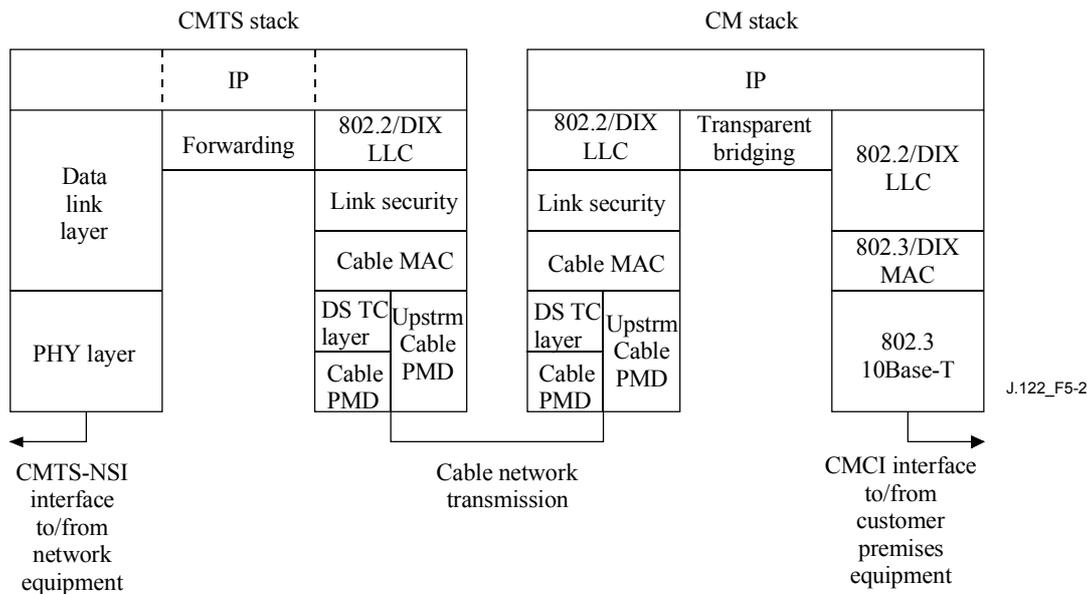
**Figure 5-2/J.122 – Data forwarding through the CM and CMTS**
