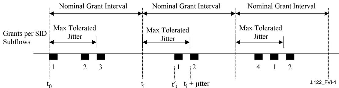
**Figure VI.1/J.122 – Example jitter with multiple grants per SID**
