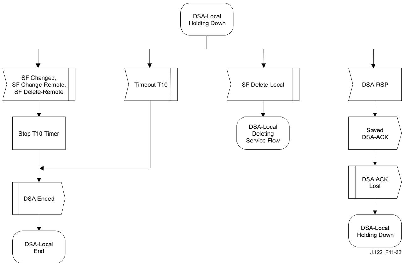
**Figure 11-33/J.122 – DSA – Locally initiated Transaction Holding State Flow Diagram**
