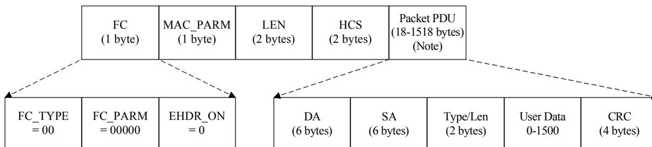
NOTE – Frame size is limited to 1518 bytes in the absence of VLAN tagging. Cooperating devices which implement IEEE 802.1Q VLAN tagging MAY use a frame size up to 1522 bytes.
