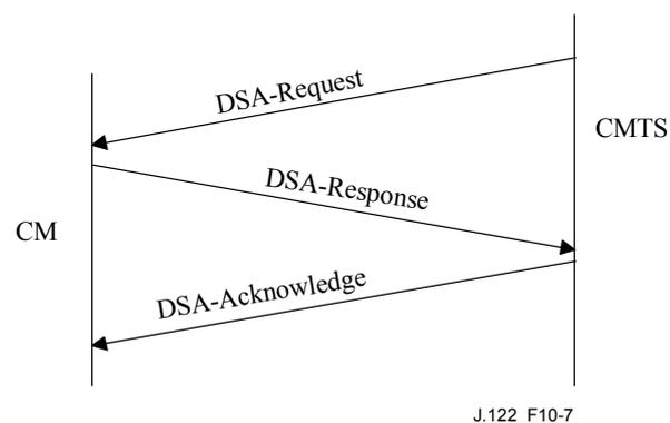
**Figure 10-7/J.122 – Dynamic Service Addition message flow – CMTS-initiated**
