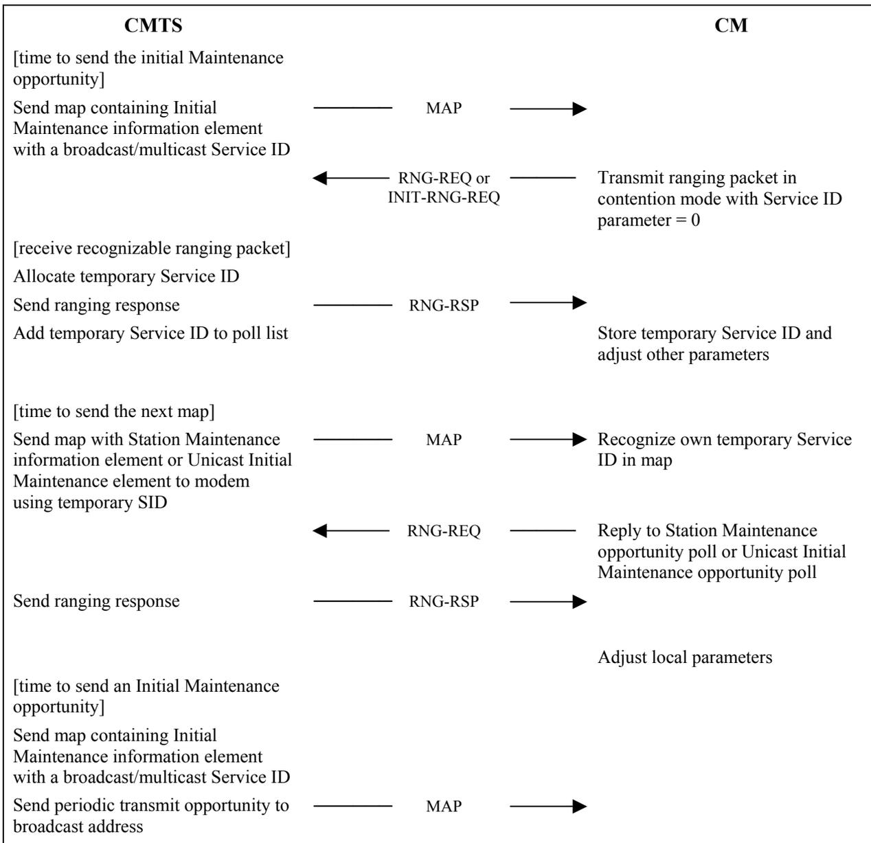
NOTE – The CMTS MUST allow the CM sufficient time to have processed the previous RNG-RSP (i.e., to modify the transmitter parameters) before sending the CM a specific ranging opportunity. This is defined as CM Ranging Response Time in Annex B.
