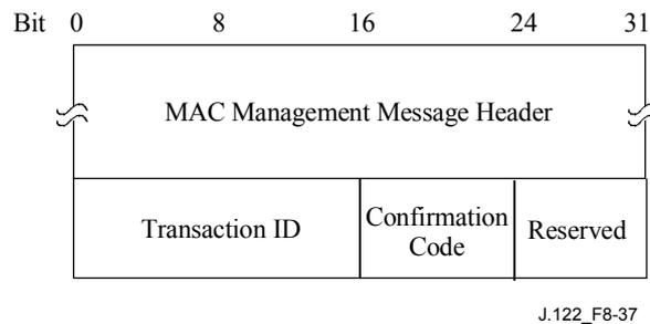
**Figure 8-37/J.122 – Dynamic Service Deletion Response**
