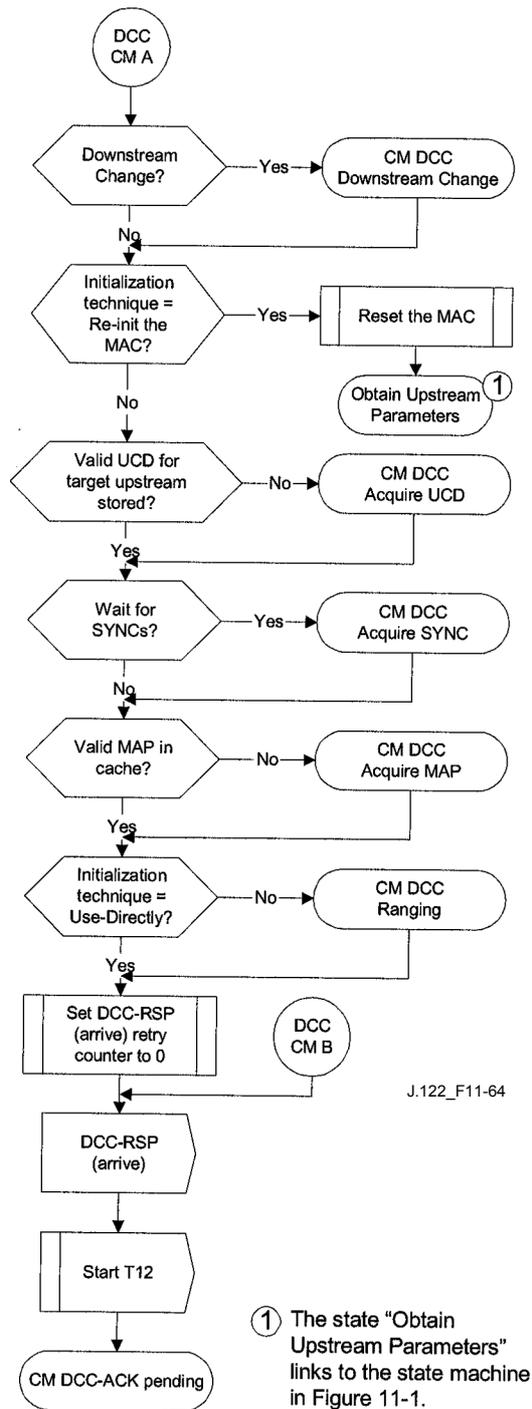
Figure 11-64/J.122 – Dynamically changing channels: CM view, Part 2
