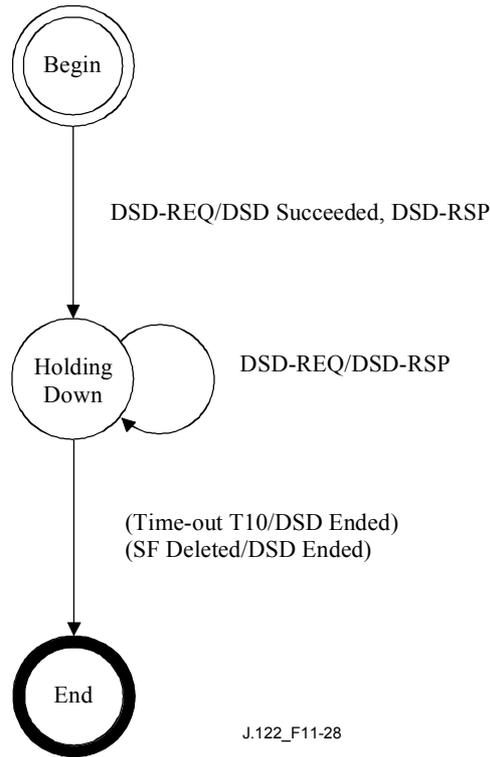
**Figure 11-28/J.122 – Dynamic Deletion (DSD) – Remotely Initiated Transaction State Transition Diagram**
