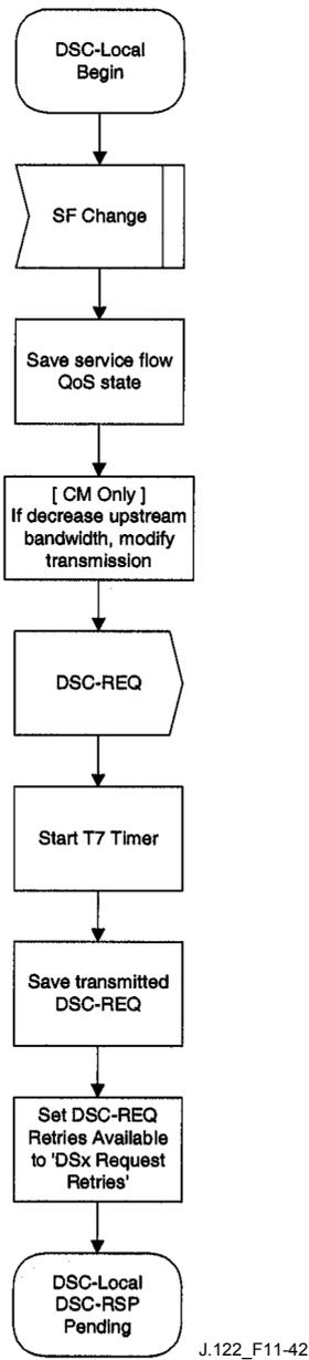
Figure 11-42/J.122 – DSC – Locally initiated Transaction DSC-RSP Pending State Flow Diagram
