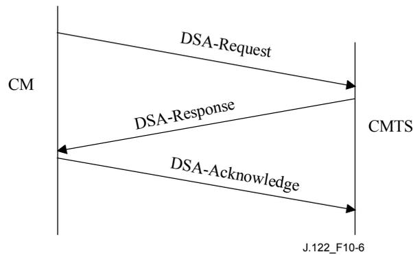
**Figure 10-6/J.122 – Dynamic Service Addition message flow – CM-initiated**
