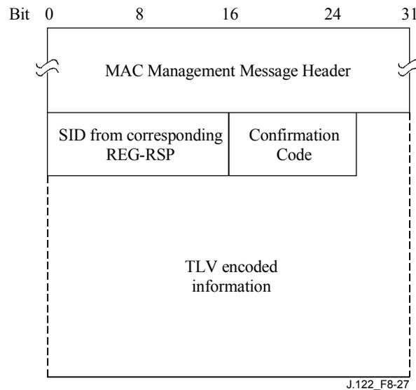
**Figure 8-27/J.122 – Registration Acknowledgment**
