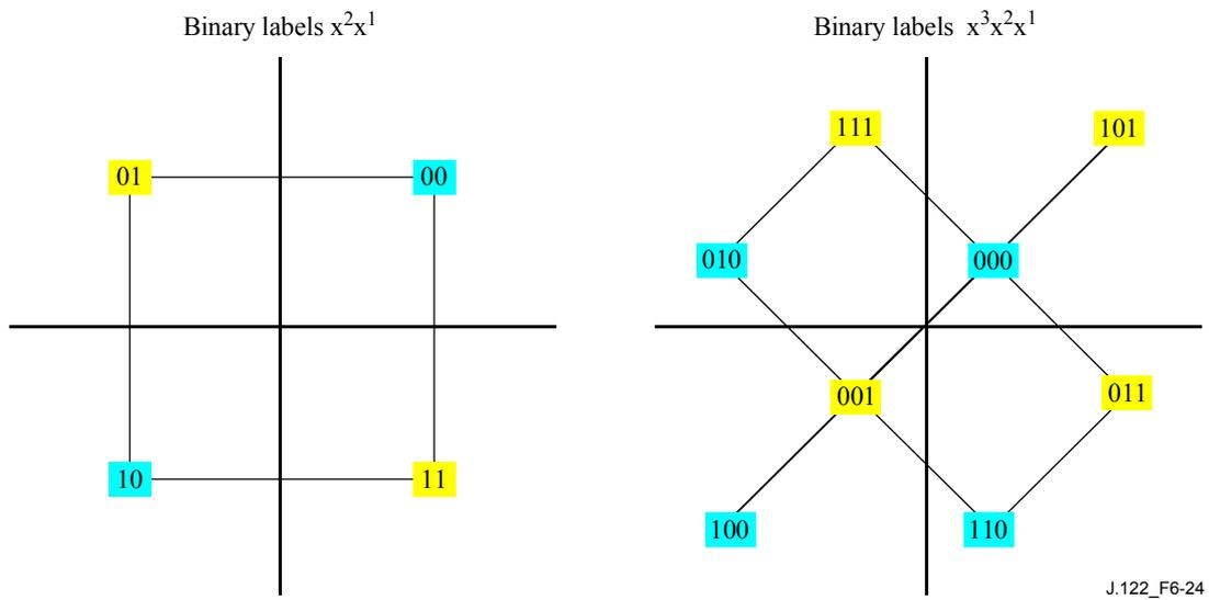
**Figure 6-24/J.122 – QPSK and 8QAM TCM symbol mapping**
