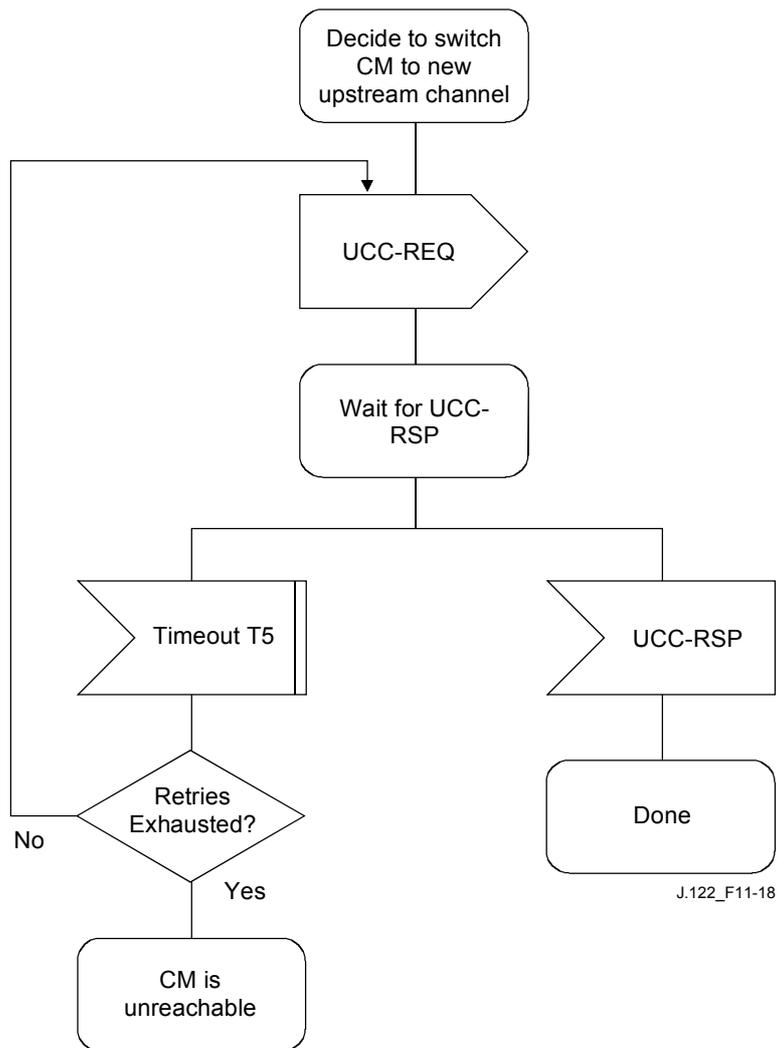
**Figure 11-18/J.122 – Changing upstream channels: CMTS view**
