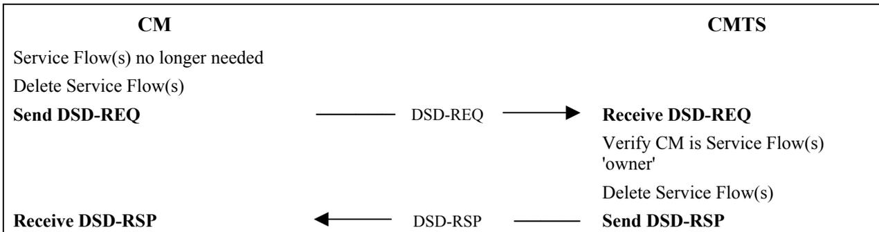
**Figure 11-51/J.122 – Dynamic Service Deletion initiated from CM**
