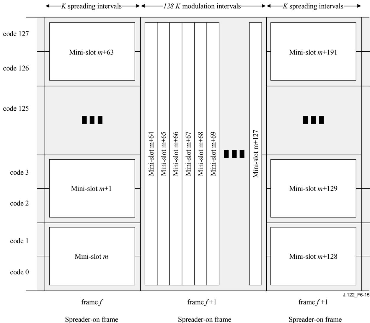
**Figure 6-15/J.122 – S-CDMA and spreader-off intervals**
