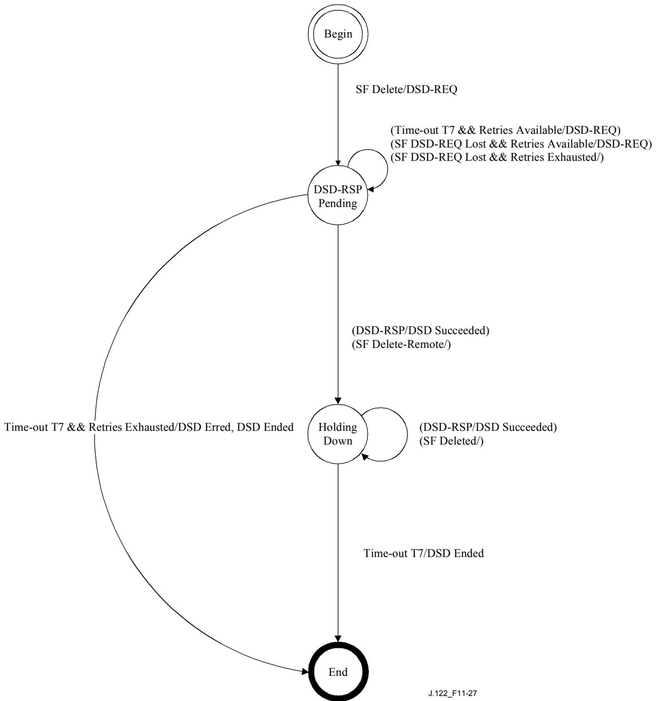
**Figure 11-27/J.122 – DSD – Locally initiated Transaction State Transition Diagram**
