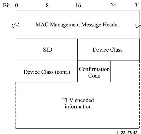
**Figure 8-42/J.122 – Device Class Identification Response**
