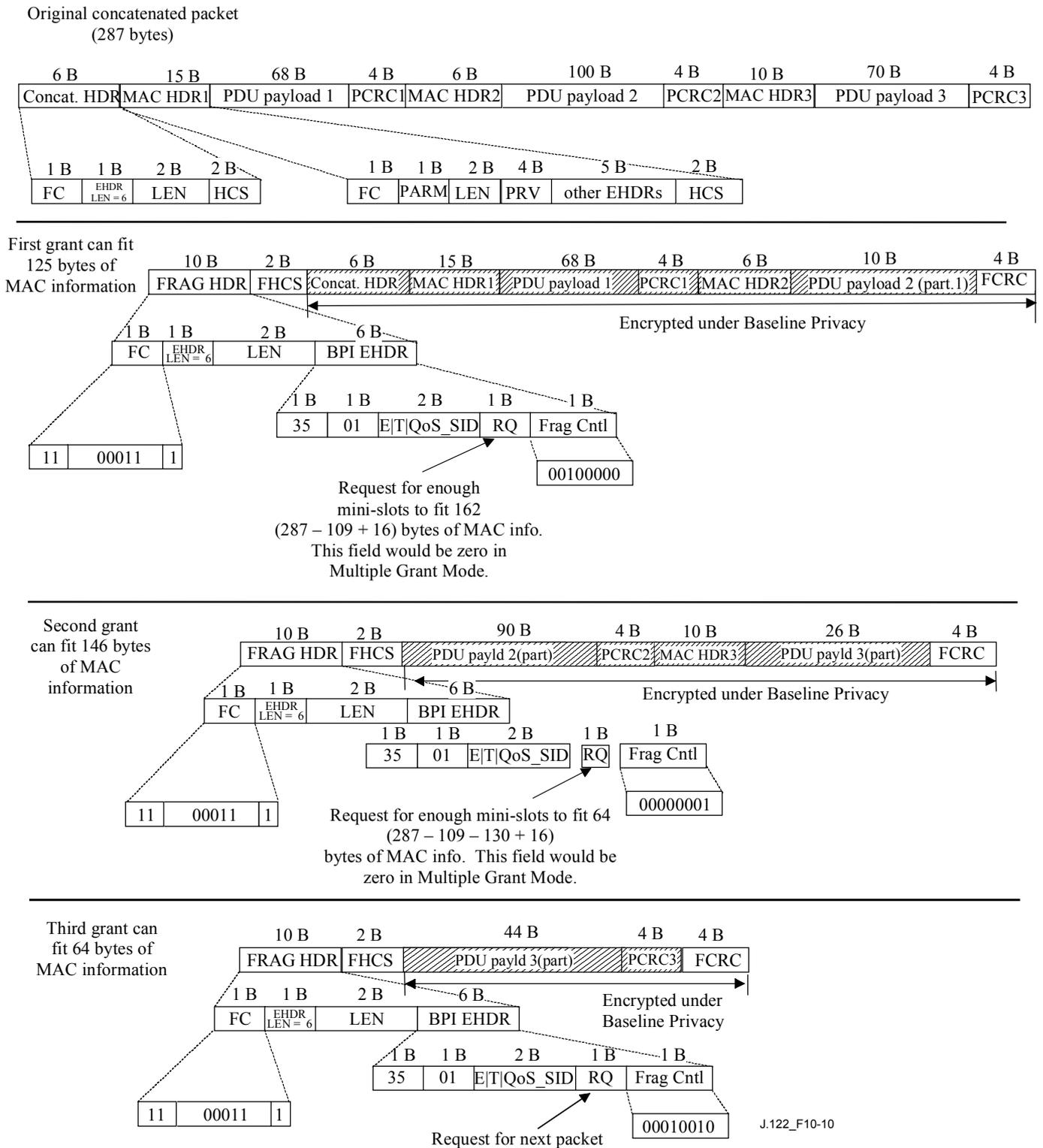
Figure 10-10/J.122 – Fragmented concatenated packet example
