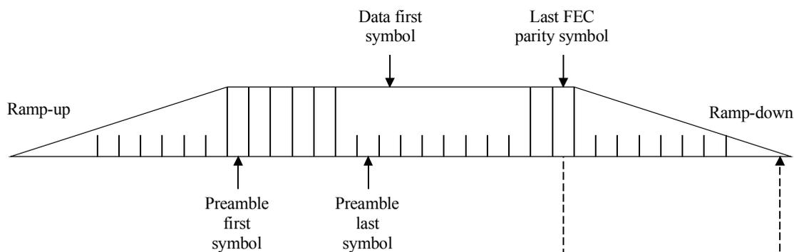
b) Timing is referenced to the symbol centre of the first symbol of each burst
