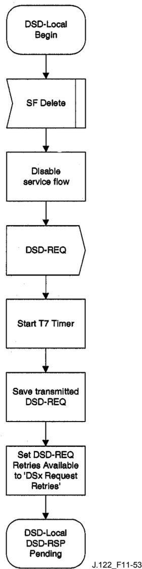
Figure 11-53/J.122 – DSD – Locally initiated Transaction Begin State Flow Diagram
