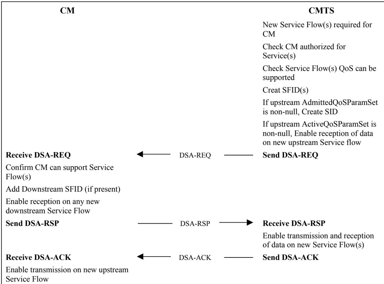
**Figure 11-30/J.122 – Dynamic Service Addition initiated from CMTS**
