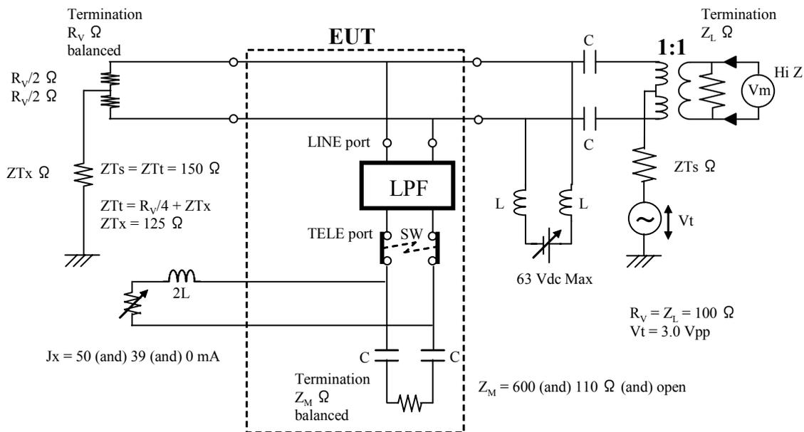
(b) VDSL band test set-up
