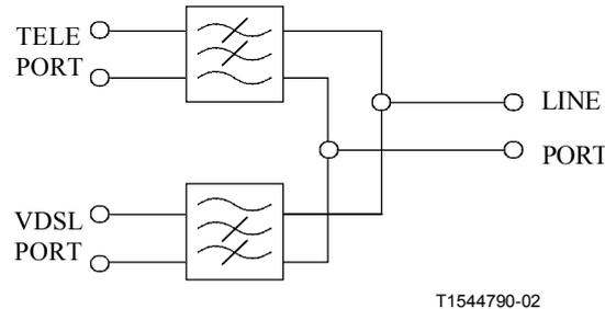
**Figure 11-1/G.993.1 – Structure of the VDSL splitter filter**
