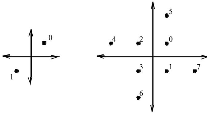
Figure 9-5: Constellation labels for  $b = 1$  and  $b = 3$
