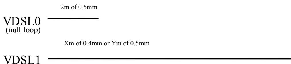
**Figure 14-1- Generic VDSL test loops**
