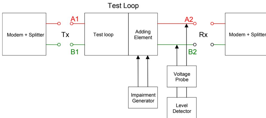
**Figure 14-5 - Functional description of the set-up of the performance tests**
