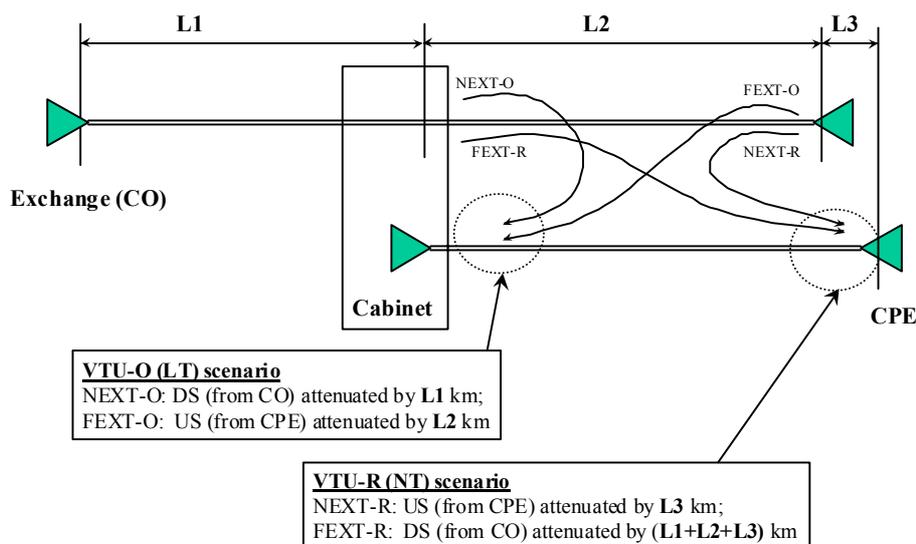
Figure 14-3 - Alien crosstalk noise model definition for different scenarios
