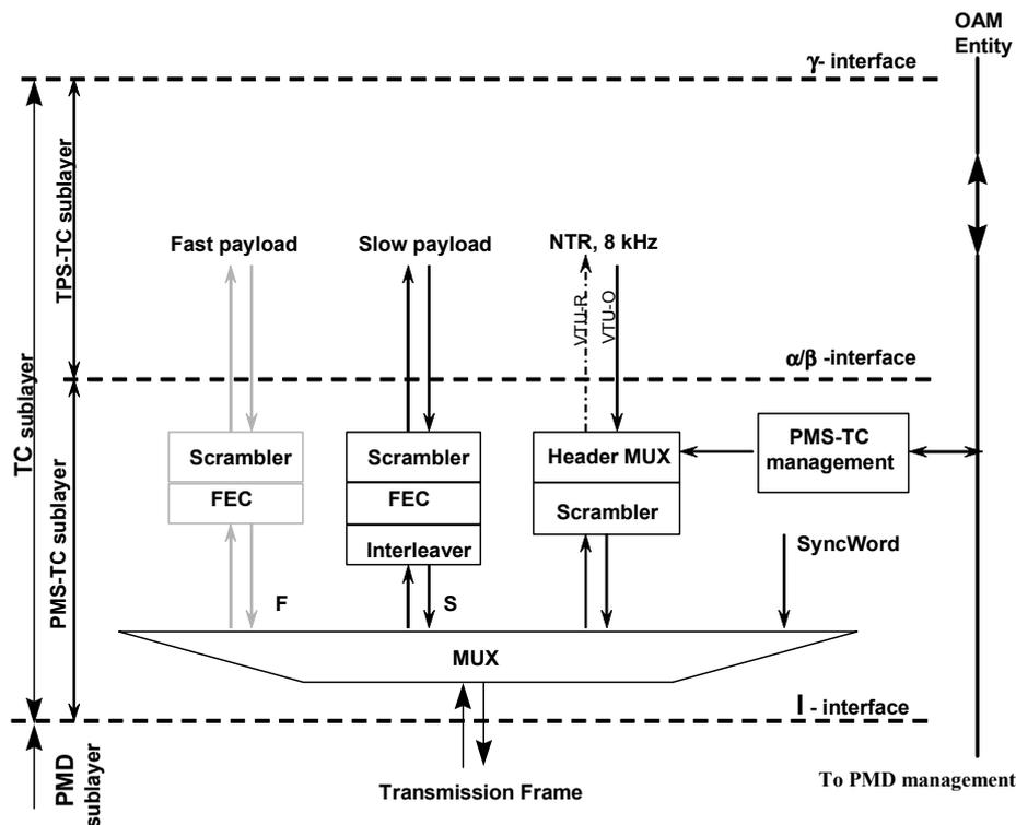
Figure I-1 - PMS-TC functional model
