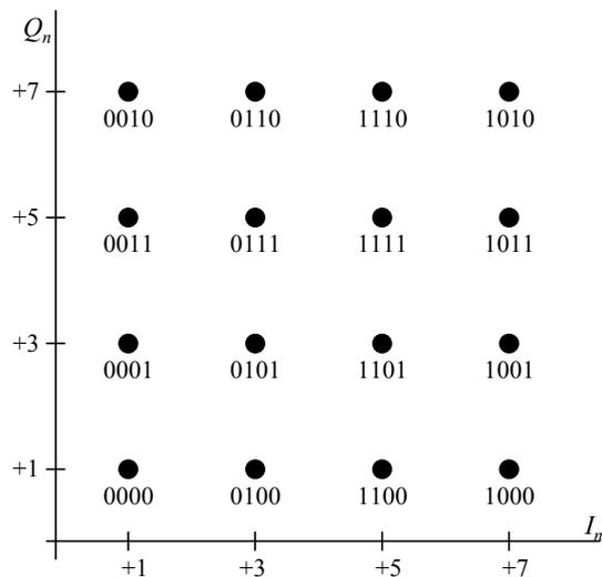
Figure I-14 - 64-point constellation and bit mapping (first quadrant)
