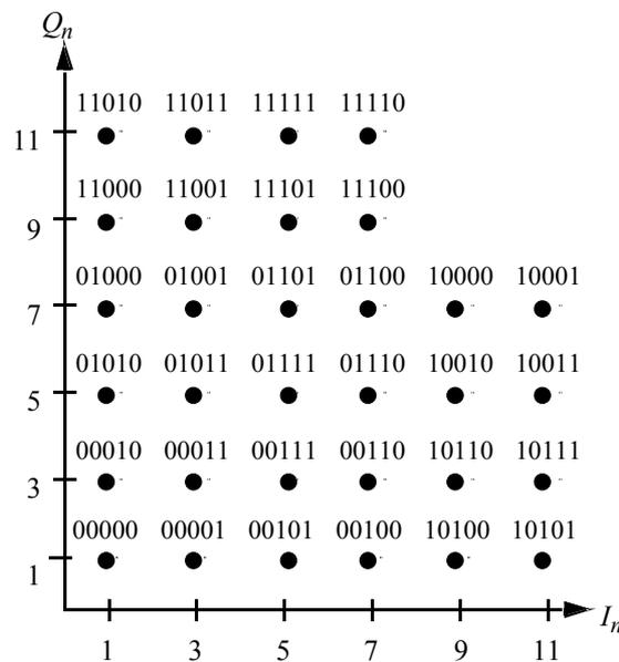
Figure I-15 - 128-point constellation and bit mapping (first quadrant)
