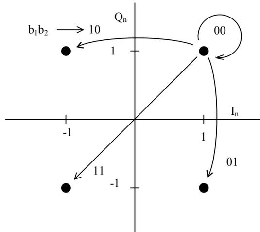
Figure I-11 - 4-point constellation with differential bit encoding
