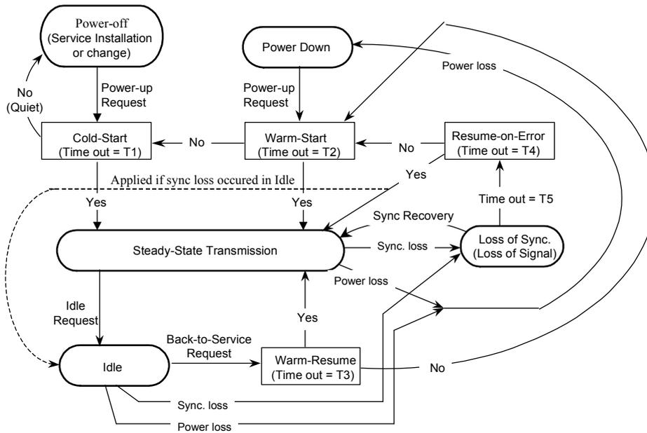
Figure I-19 - VDSL link state and timing diagram
