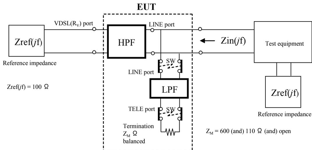
(b) VDSL band test set-up
