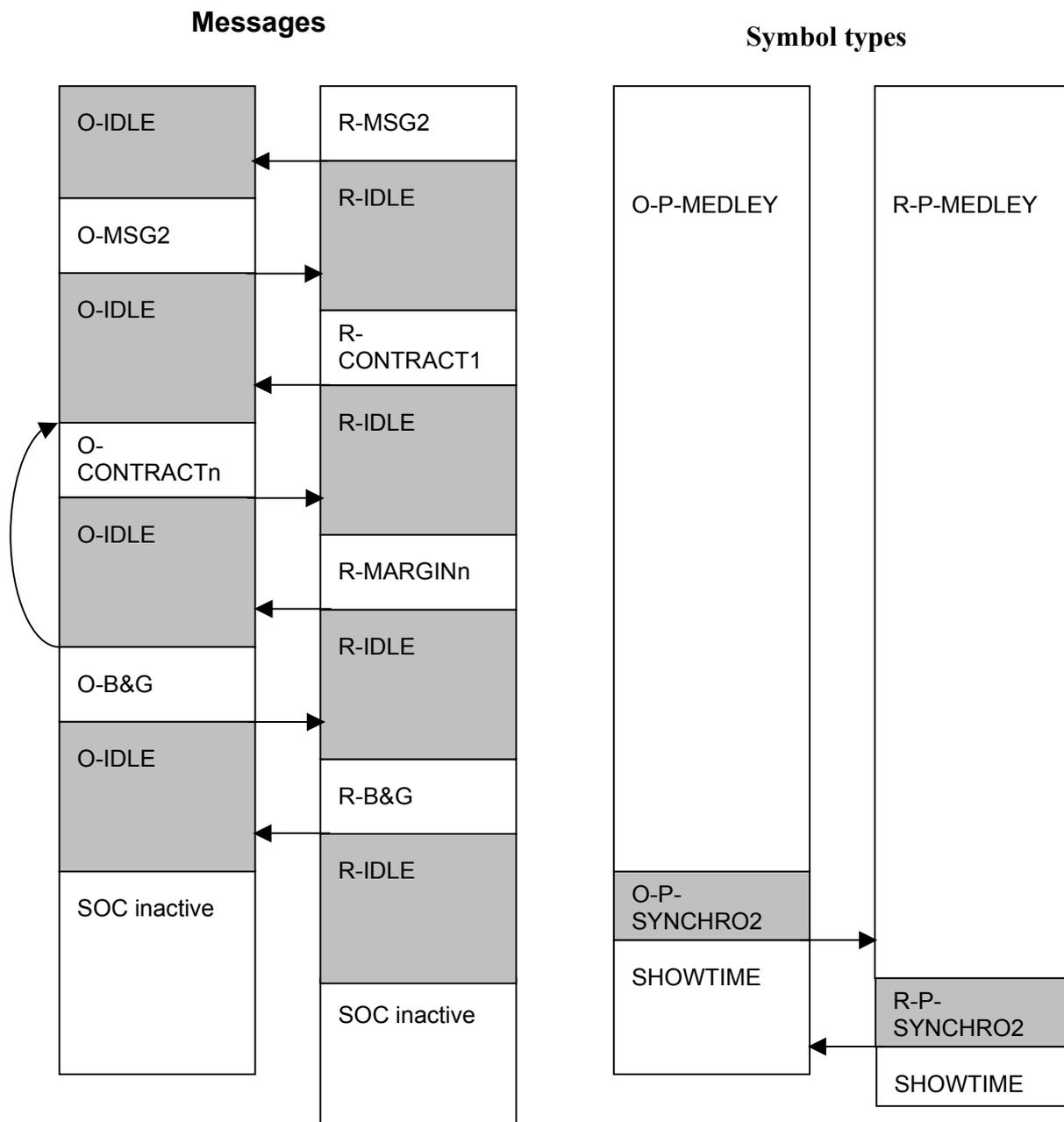
Figure 12-7: Timeline of the channel analysis and exchange phase
