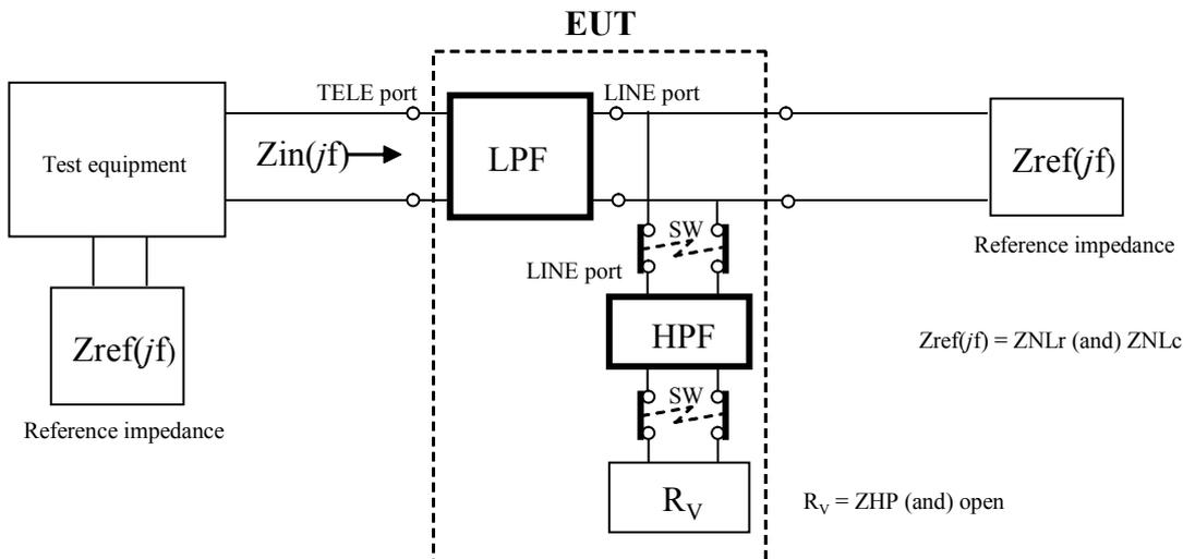
(a) Voice band test set-up
