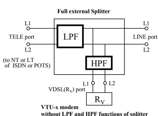
(c) Type J2: Full internal LPF and HPF splitter      (d) Type J3: Full external LPF and HPF splitter
