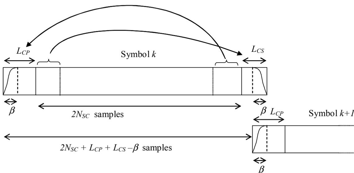
Figure 9-2: Cyclic extensions, windowing and overlap of DMT symbols
