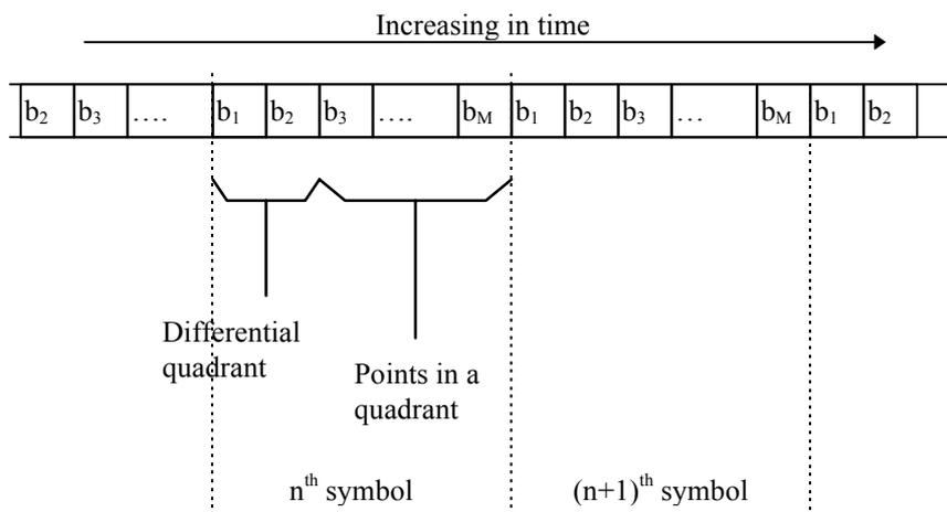
Figure I-10 - Bit to symbol mapping
