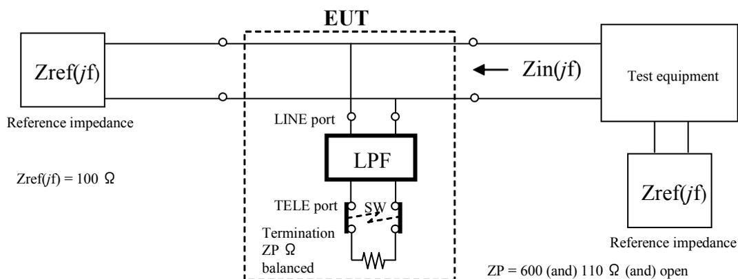
**(c) VDSL band test set-up**
