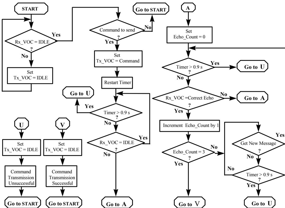
Figure I-17 - VTU-O VOC handshaking flow chart
