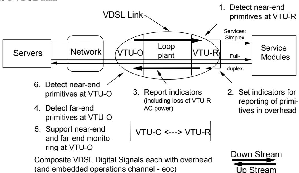
**Figure 10-4: In-service surveillance of the VDSL link shown from the VTU-O's standpoint**
