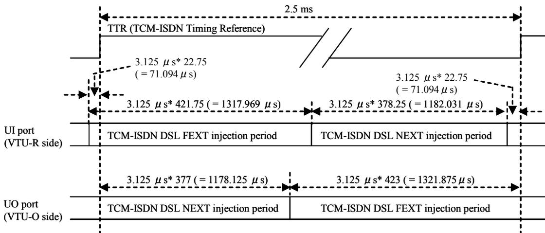
**Figure F-16/G.993.1 – TCM-ISDN DSL alternate NEXT and FEXT injection timing**
