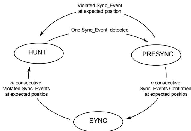
Figure I-26 - Frame delineation state machine
