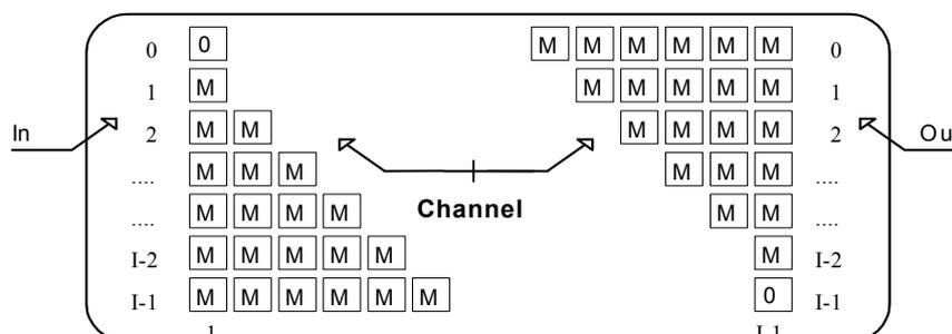
**Figure I-27 - Interleaver/de-interleaver implementation example**
