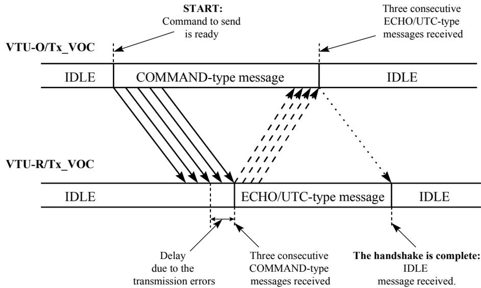
**Figure I-16 - Example of VOC handshake for a successfully communicated command**
