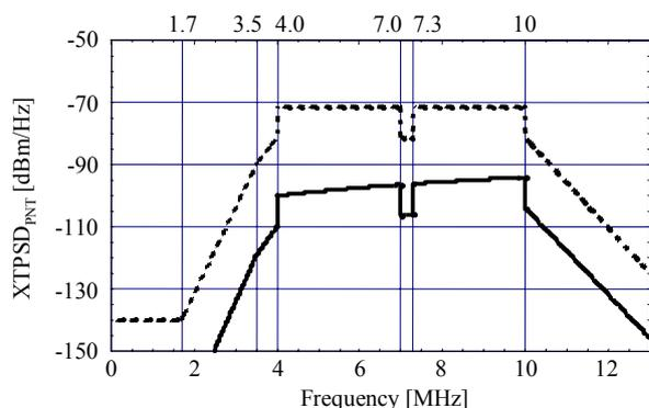
Figure F-15/G.993.1 – 9-disturber PNT NEXT PSD for injection at UI and UO ports
