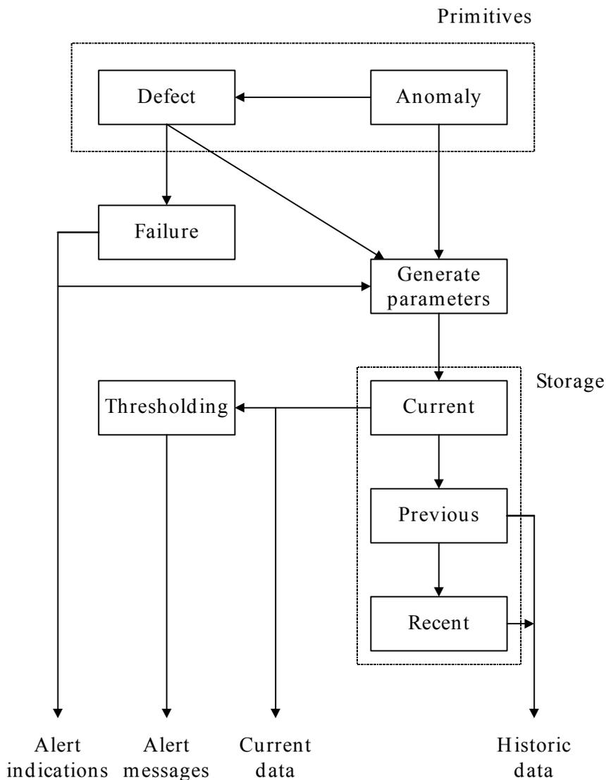
**Figure 10-3: Performance monitoring process**
