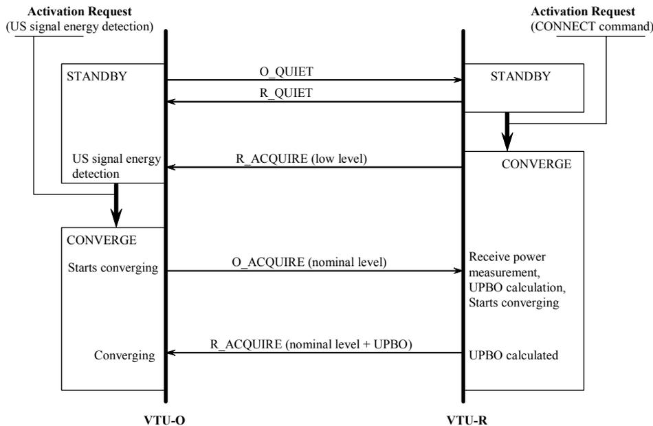
**Figure I-25 - Activation from the VTU-R**
