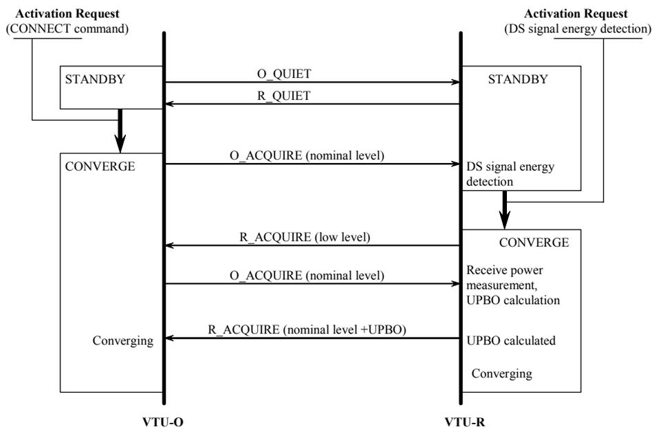
Figure I-24 - Activation from the VTU-O
