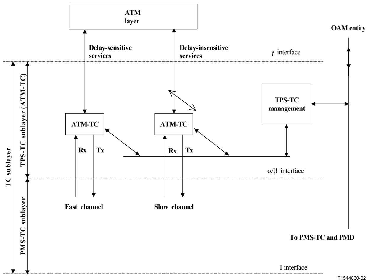
NOTE – At VTU-O: Tx = Downstream, Rx = Upstream. At VTU-R: Tx = Upstream, Rx = Downstream
