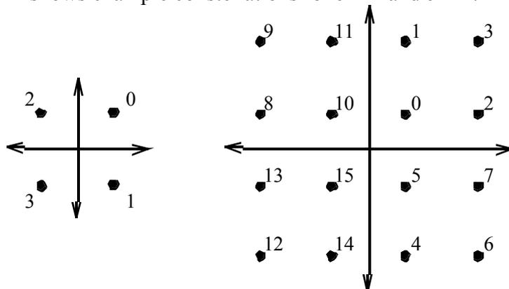
Figure 9-4: Constellation labels for  $b = 2$  and  $b = 4$
