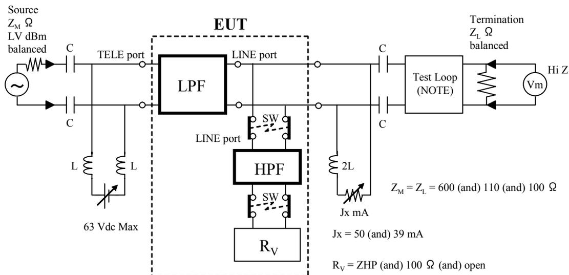
NOTE – Test loop is used only for voice band test. Null loop is applied for ISDN and VDSL band test.
