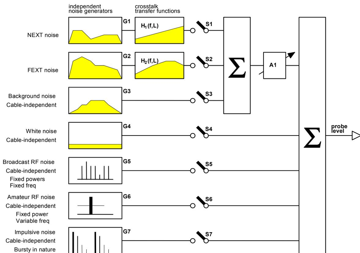
**Figure 14-2 - Functional diagram of the composition of the impairment noise**
