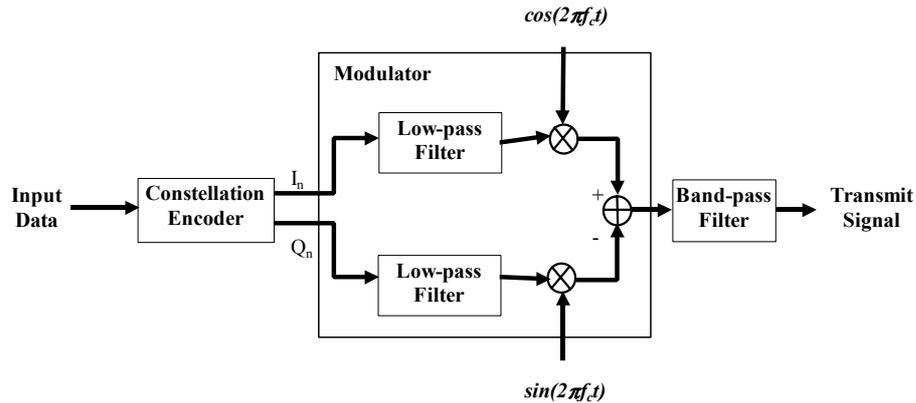
Figure I-9 - Block diagram of a SCM transmitter
