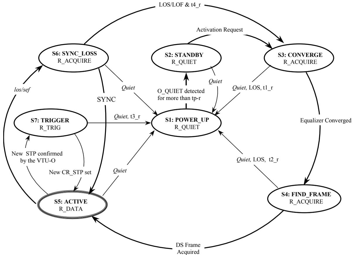
Figure I-23 - VTU-R activation/deactivation state machine
