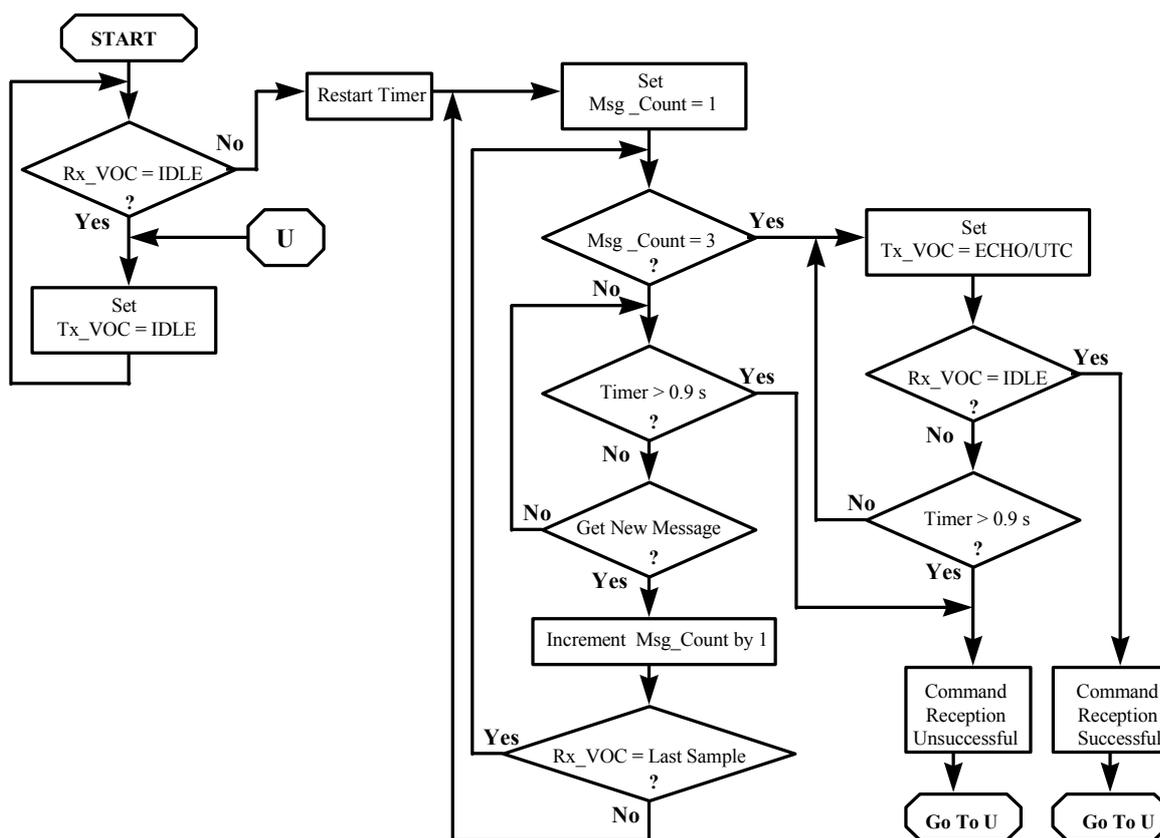
Figure I-18 - VTU-R VOC handshaking flow chart
