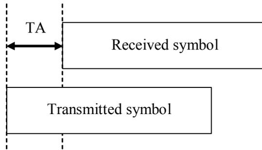
**Figure 9-3: Illustration of Timing Advance (TA)**
