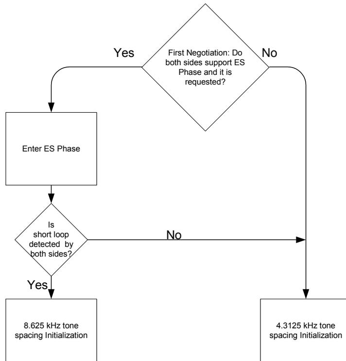
**Figure IV-2: Flow chart of the 8.625 kHz tone spaced initialization**
