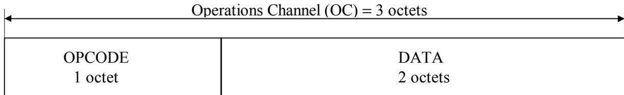
**Figure I-5 - Operations channel field**
