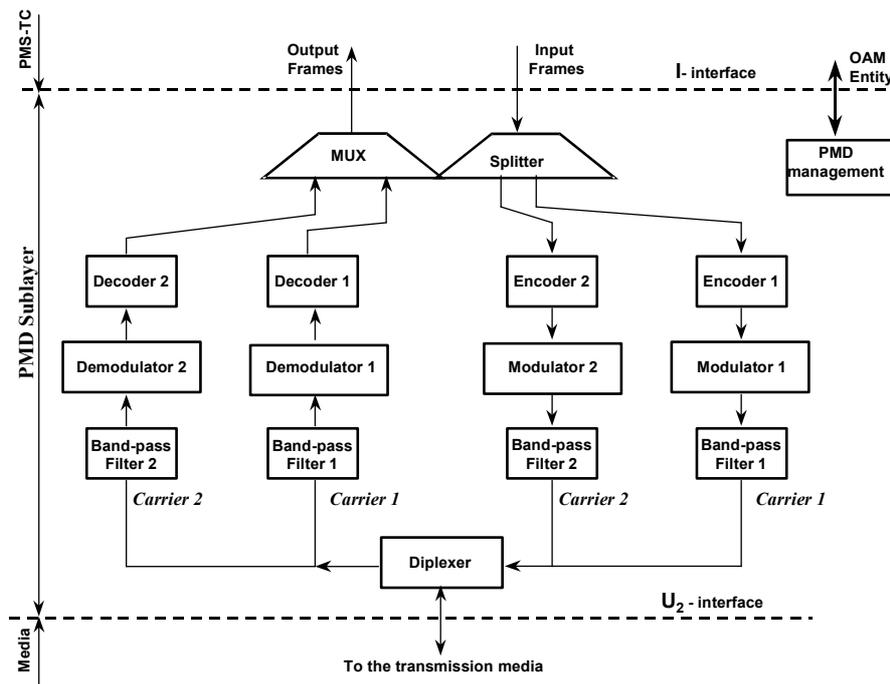
Figure I-7 - VTU PMD sublayer functional model
