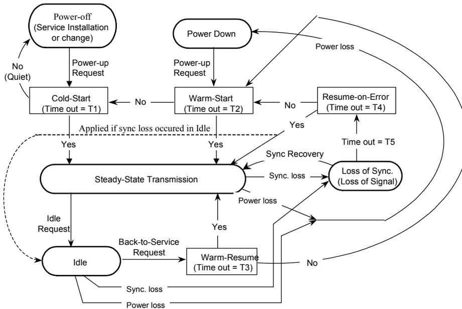
Figure 12-1: VDSL link state and timing diagram
