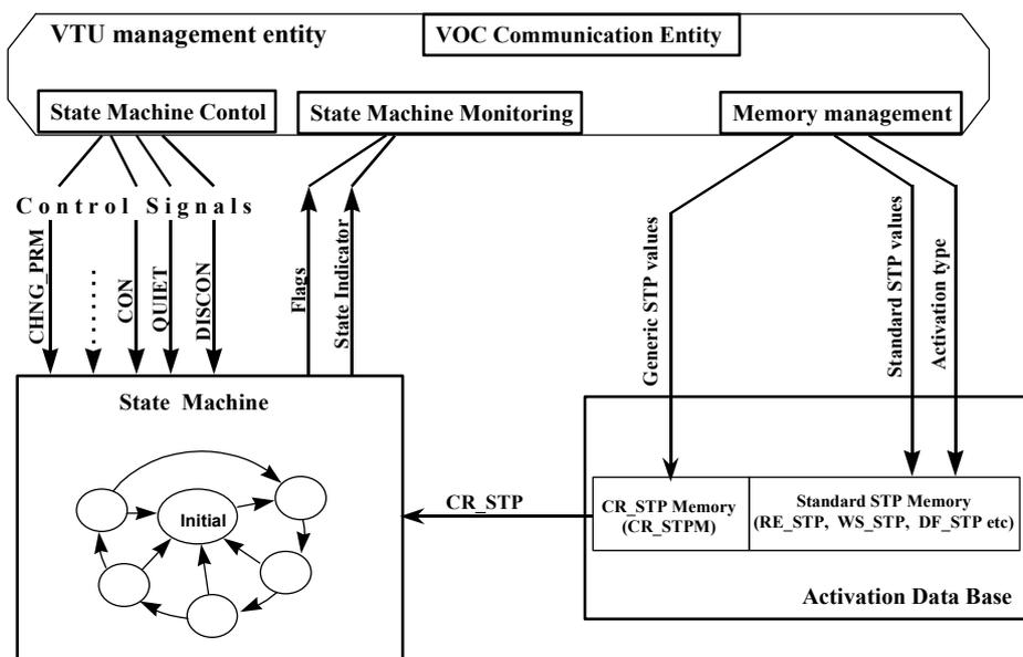
Figure I-20 - VTU- activation/deactivation functional diagram
