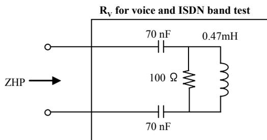
Figure F-2/G.993.1 – ZHP definition as  $R_V$  for voice and ISDN band test
