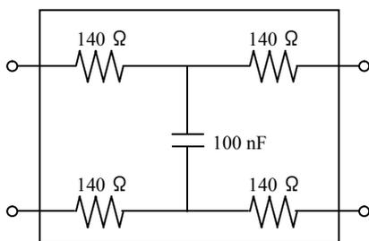
**Figure F-4/G.993.1 – Voice band test loop (approx. 2 km)**
