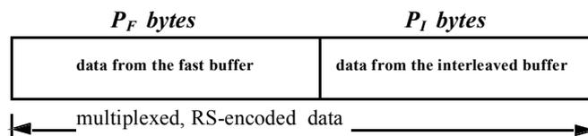
Figure 8-4: Convergence of the fast and interleaved data into one frame
