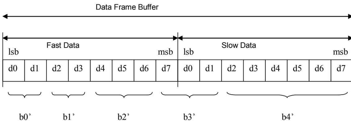
**Figure 9-7: Bit extraction after tone ordering**
