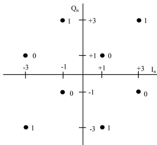
**Figure I-12 - 8-point constellation and bit mapping**
