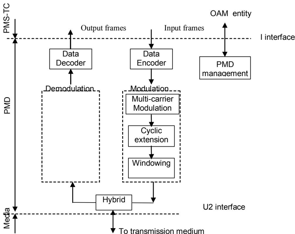
Figure 9-1: Functional diagram of PMD sublayer
