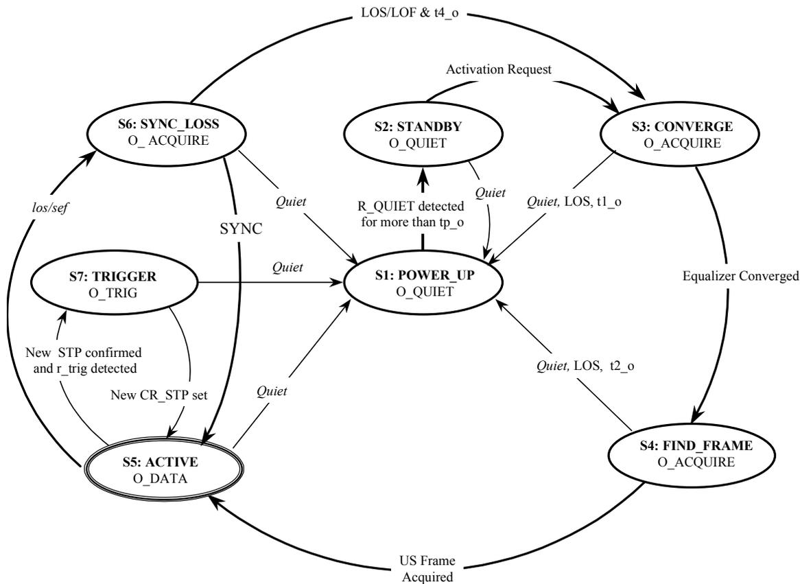
Figure I-21 - VTU-O activation/deactivation state machine
