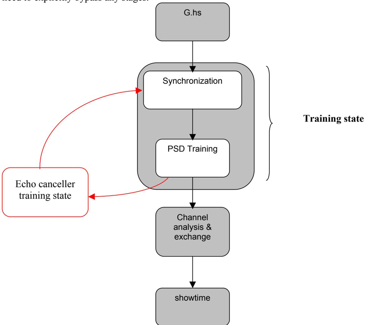
Figure 12-6: Position of (optional) echo canceller training state in the initialization procedure
