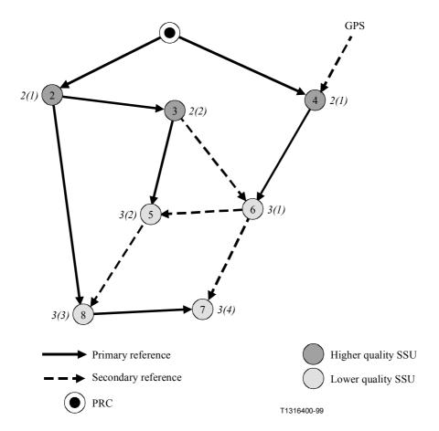
Figure III.3a/G.803 – Successful N(m) labelling of SSUs: No potential timing loops
