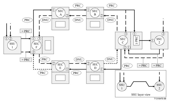
Figure III.9/G.803 – SDH ring network with filtering SSU
