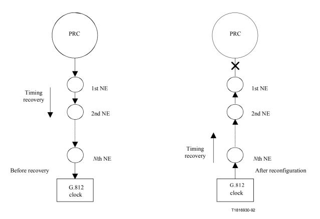
**Figure 8-6/G.803 – Reconfiguration example**
