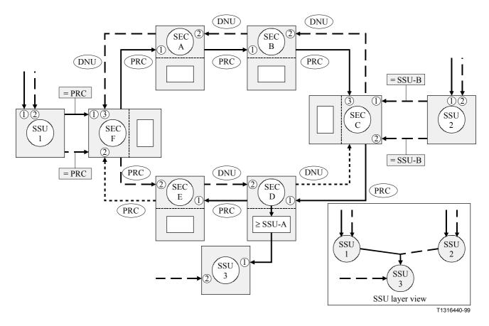
Figure III.6/G.803 – SDH ring network with two source SSUs and one sink SSU
