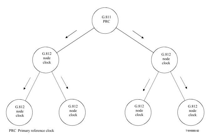
Figure 8-2/G.803 – Synchronization network architecture inter-node distribution
