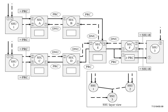
Figure III.7/G.803 – SDH Y-network with two source SSUs and one sink SSU
