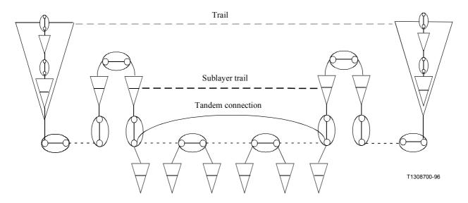
Figure 6-1/G.803 – Tandem connection monitoring by means of a sublayer trail
