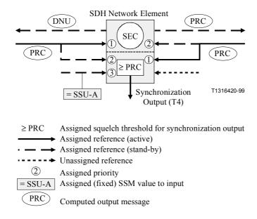
Figure III.4/G.803 – Conventions used in SEC subnetwork drawings
