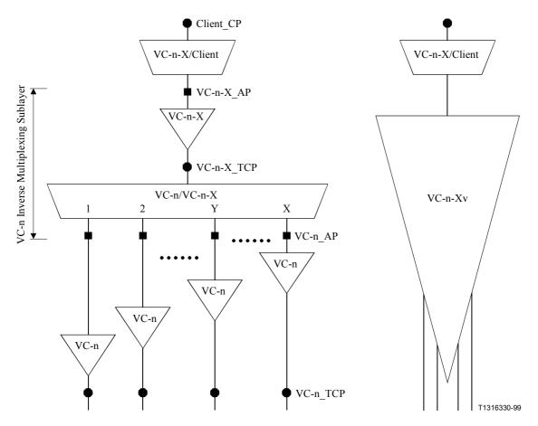
Figure 5-5b/G.803 – Inverse multiplexing/virtual concatenation model
