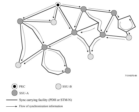
Figure III.1b/G.803 – SSU-Level constructed from Figure III.1a/G.803
