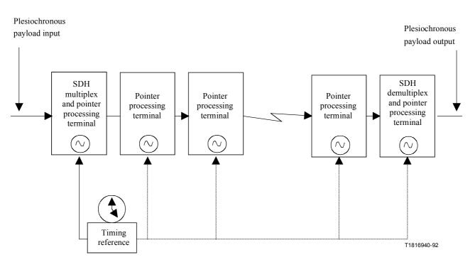
Figure 8-7/G.803 – SDH network model for pointer activity simulation
