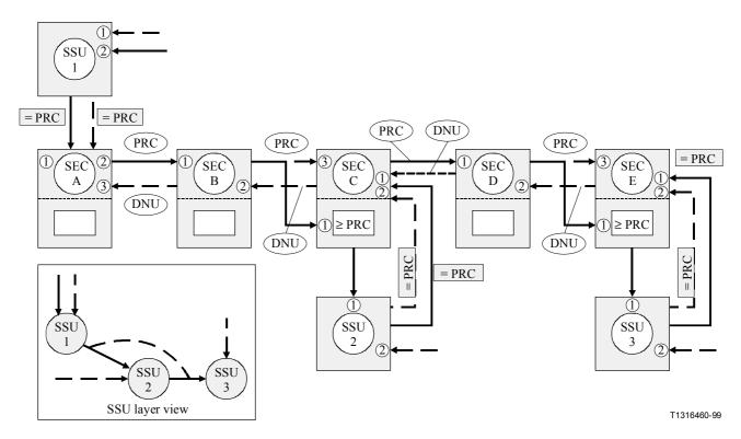
Figure III.8/G.803 – SDH linear network with filtering SSUs
