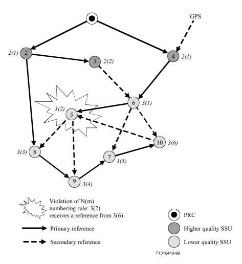
Figure III.3b/G.803 – N(m) labelling is not possible: Potential timing loop(s)
