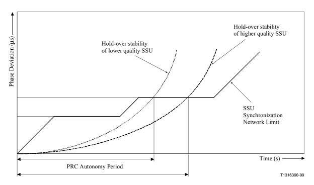
Figure III.2/G.803 – Determining the PRC Autonomy Period of an SSU
