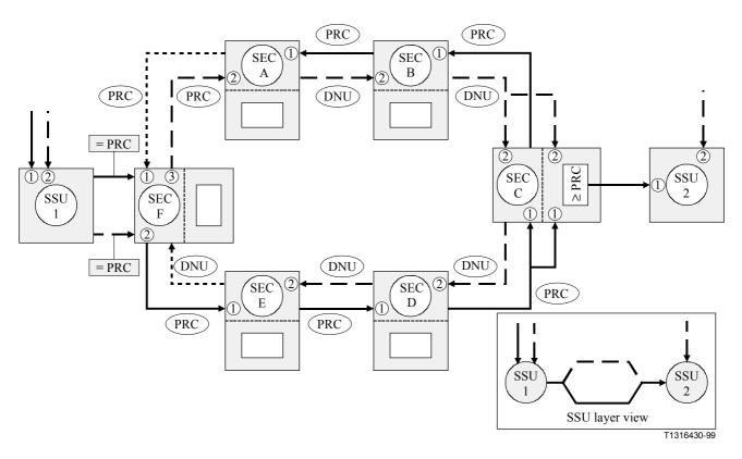
Figure III.5/G.803 – SDH ring network with one source SSU source and one sink SSU
