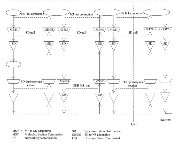
Figure 8-4/G.803 – Example of synchronization distribution across a PDH UNI
