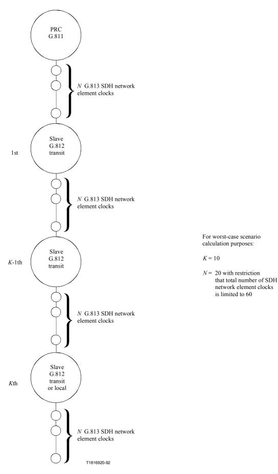
Figure 8-5/G.803 – Synchronization network reference chain
