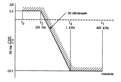
*Note 1* - The frequency  $f_0$  should be less than 20 Hz and as low as possible (e.g. 10 Hz), taking into account the limitations of measuring equipment.
