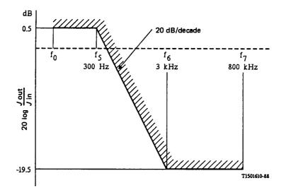
Note 1 - The frequency  $f_0$  should be less than 20 Hz and as low as possible (e.g. 10 Hz), taking into amount the limitations of measuring equipment.
